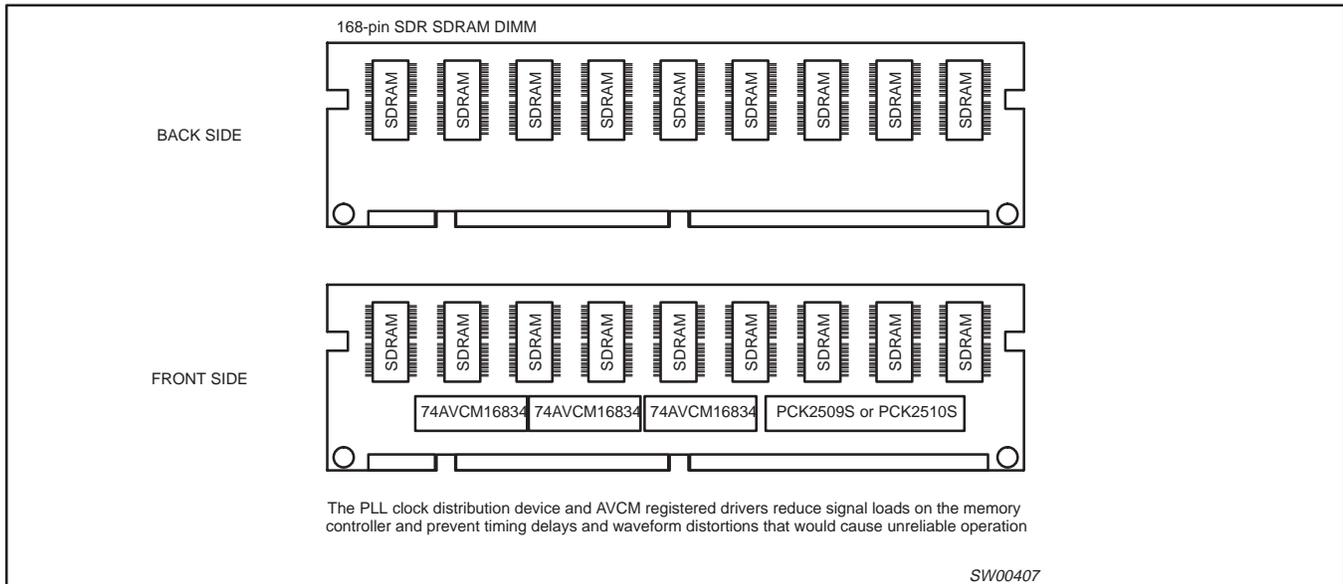
The PLL clock distribution device and AVCM registered drivers reduce signal loads on the memory controller and prevent timing delays and waveform distortions that would cause unreliable operation
