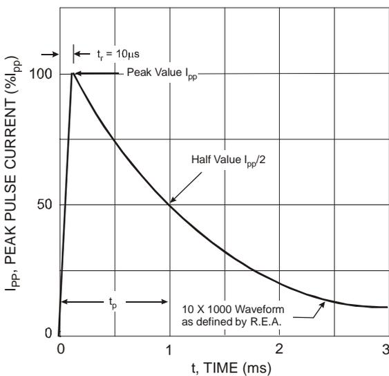
Figure 1 Pulse Waveform
