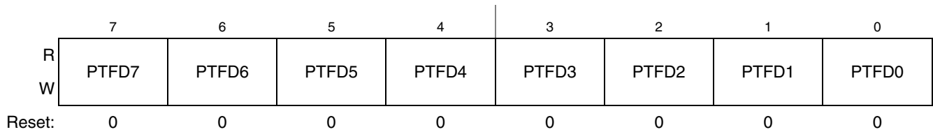
Figure 6-31. Port F Data Register (PTFD)
