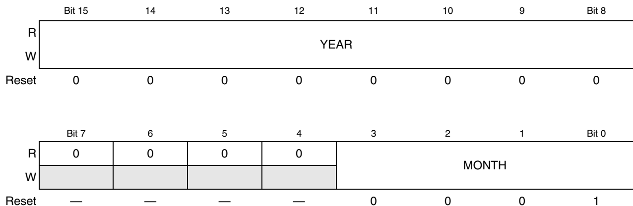
Figure 16-2. IRTC Year & Month Counters (IRTC_YEARMON) Register
