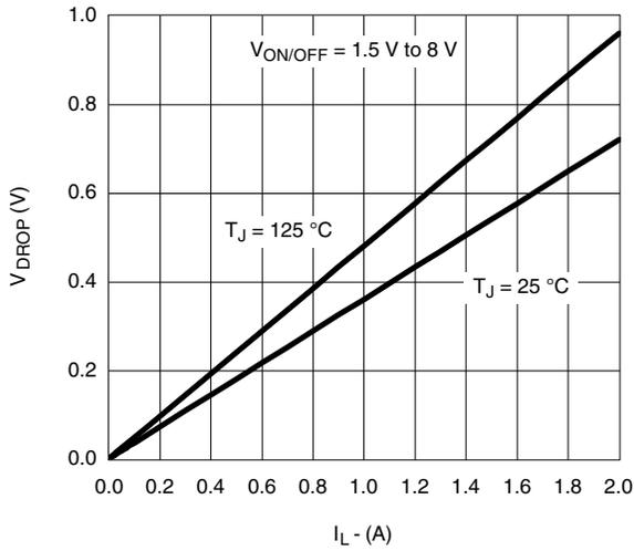
**V<sub>DROP</sub> vs. I<sub>L</sub> at V<sub>IN</sub> = 4.5 V**
