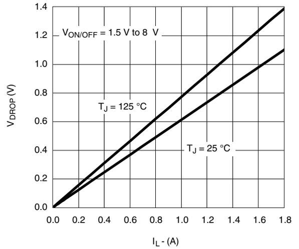
**V<sub>DROP</sub> vs. I<sub>L</sub> at V<sub>IN</sub> = 2.5 V**
