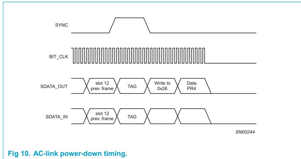
**Fig 10. AC-link power-down timing.**
