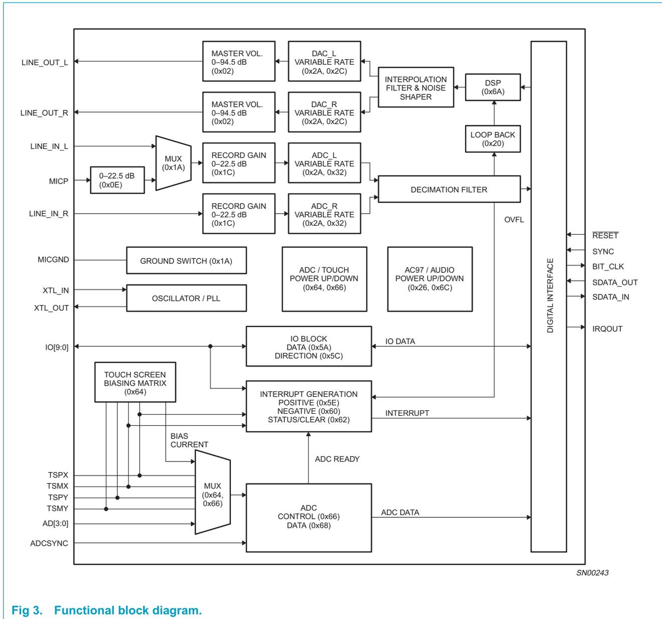
Fig 3. Functional block diagram.
