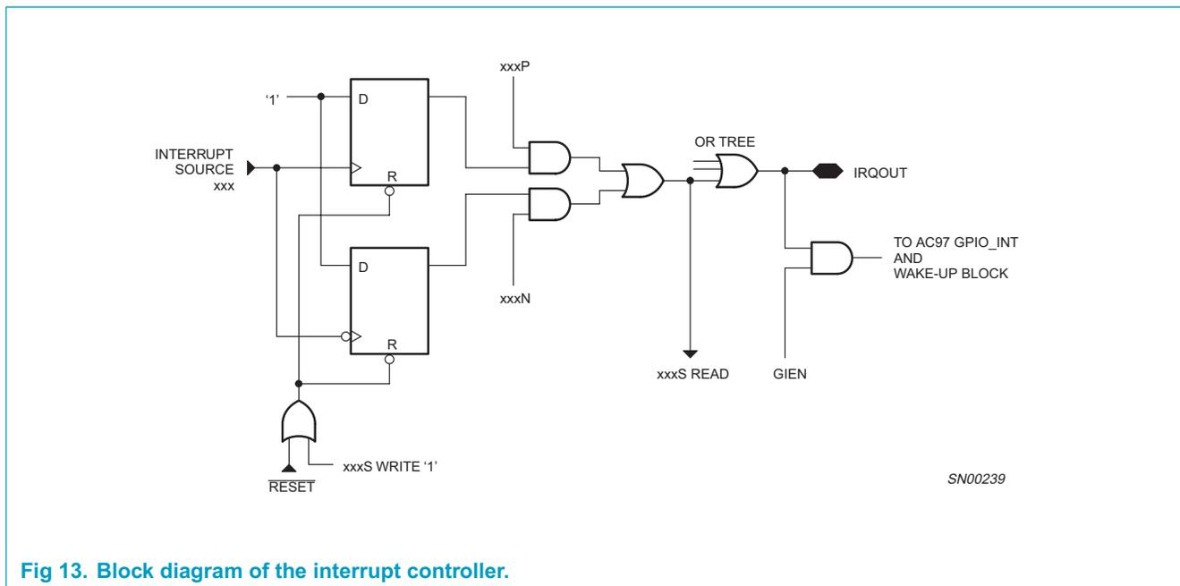
Fig 13. Block diagram of the interrupt controller.
