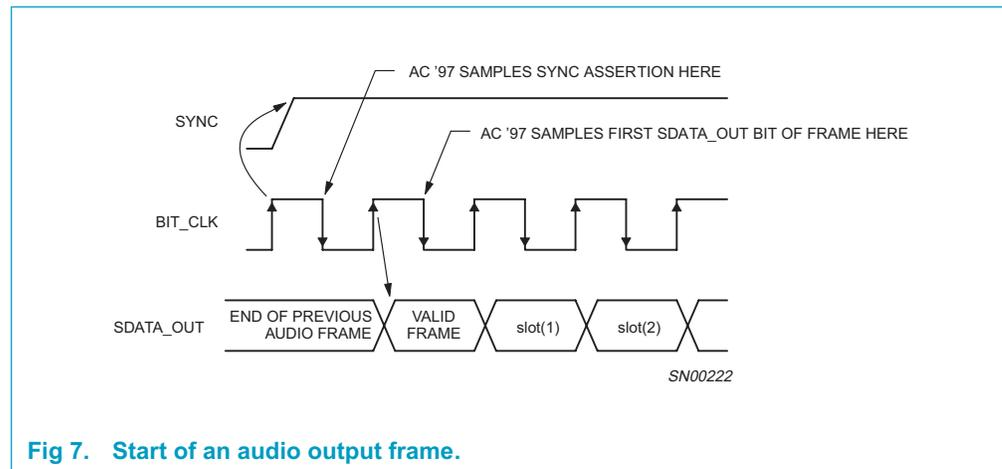
**Fig 7. Start of an audio output frame.**
