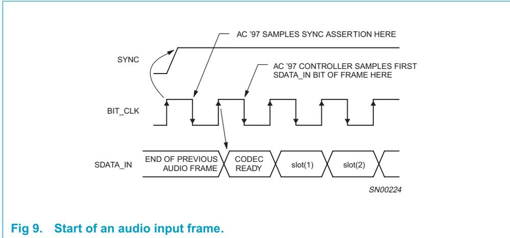
Fig 9. Start of an audio input frame.
