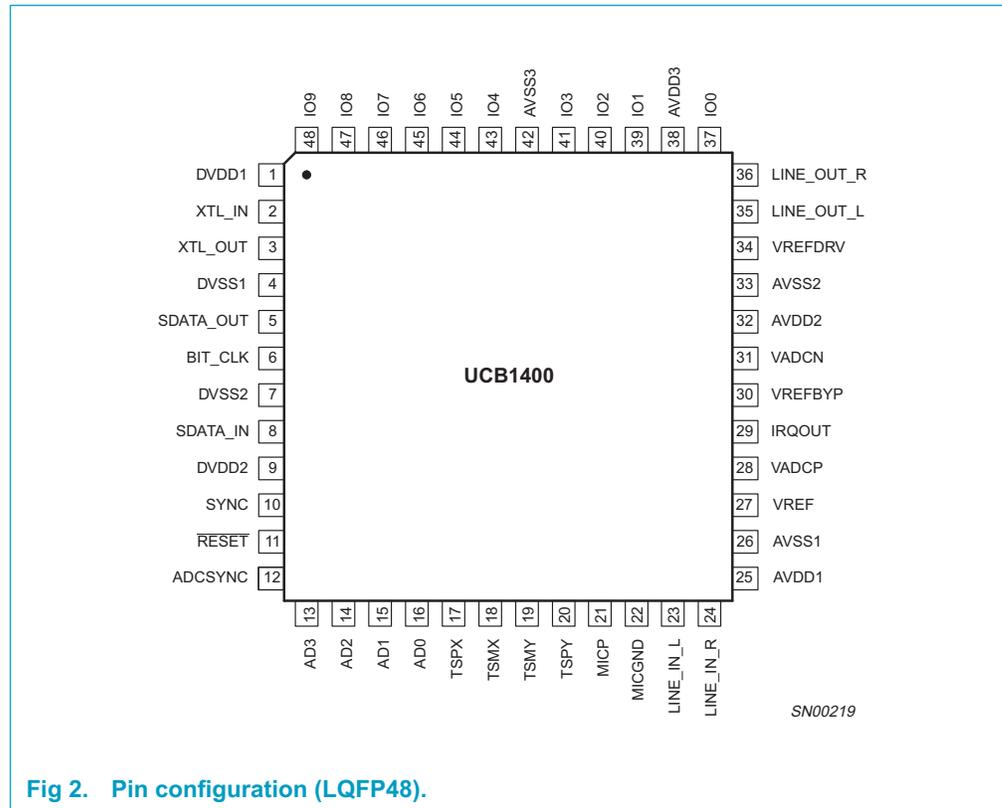
Fig 2. Pin configuration (LQFP48).
