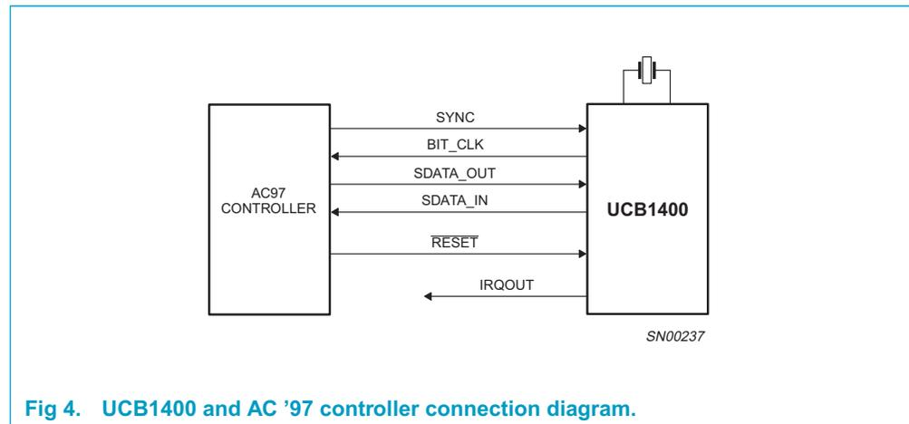
Fig 4. UCB1400 and AC '97 controller connection diagram.
