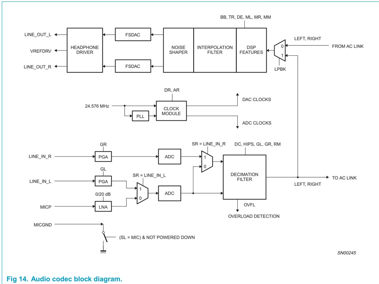
Fig 14. Audio codec block diagram.
