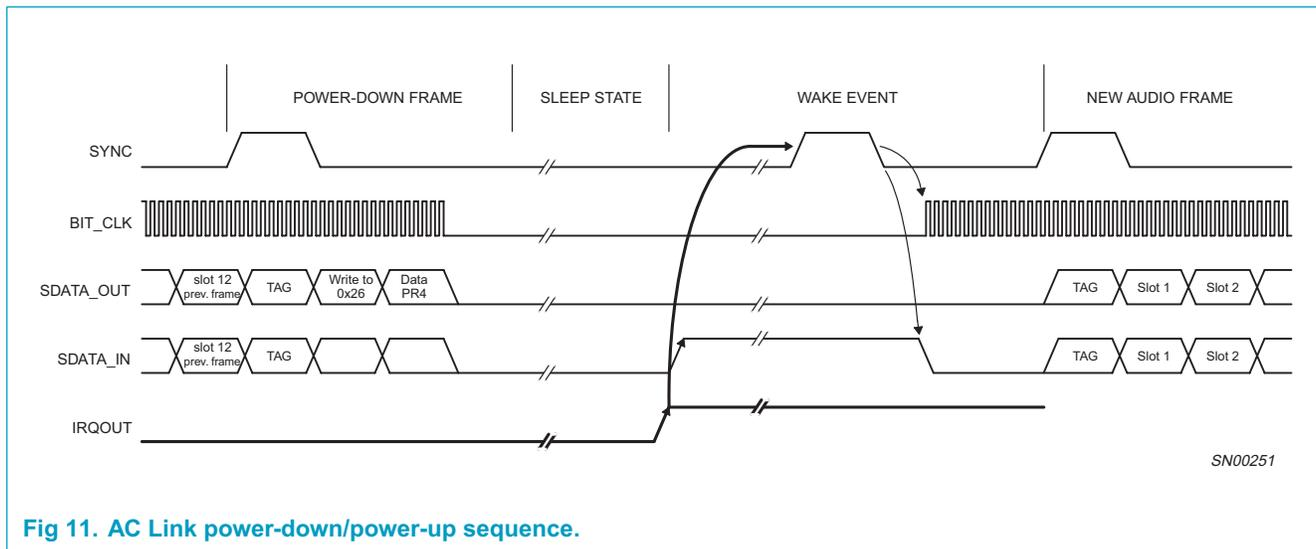
Fig 11. AC Link power-down/power-up sequence.
