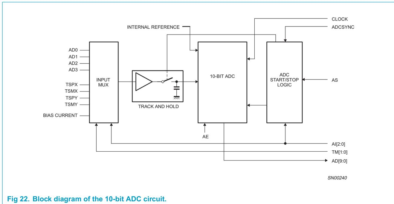
Fig 22. Block diagram of the 10-bit ADC circuit.
