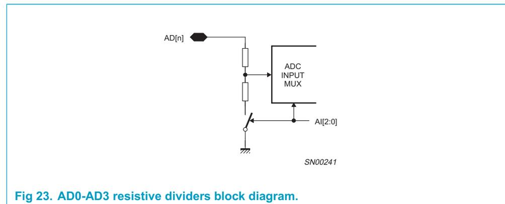
Fig 23. AD0-AD3 resistive dividers block diagram.
