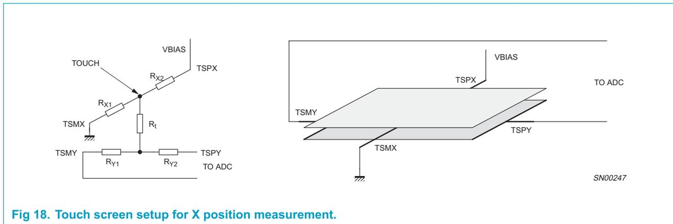
Fig 18. Touch screen setup for X position measurement.
