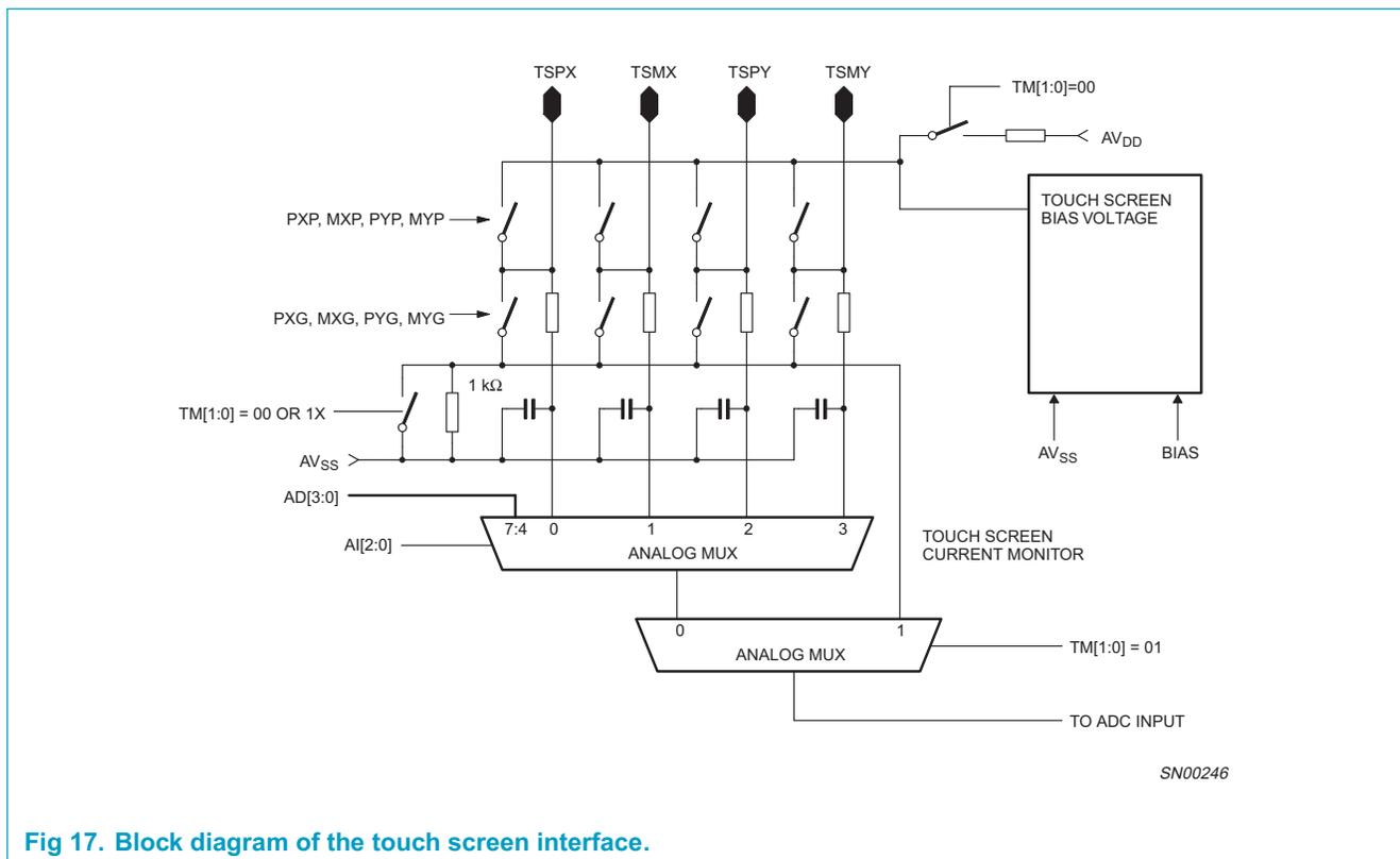
Fig 17. Block diagram of the touch screen interface.
