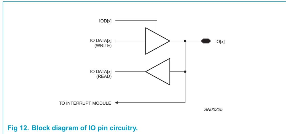
Fig 12. Block diagram of IO pin circuitry.
