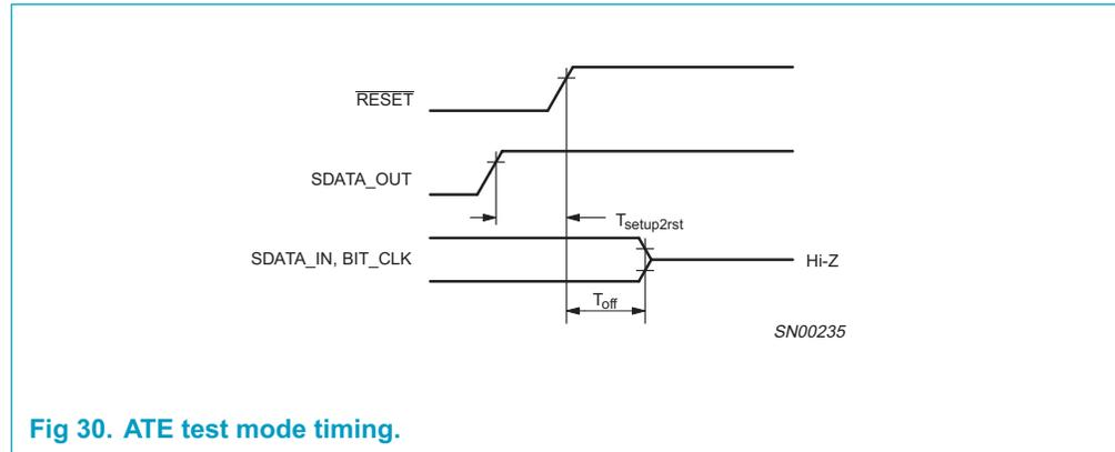
Fig 30. ATE test mode timing.
