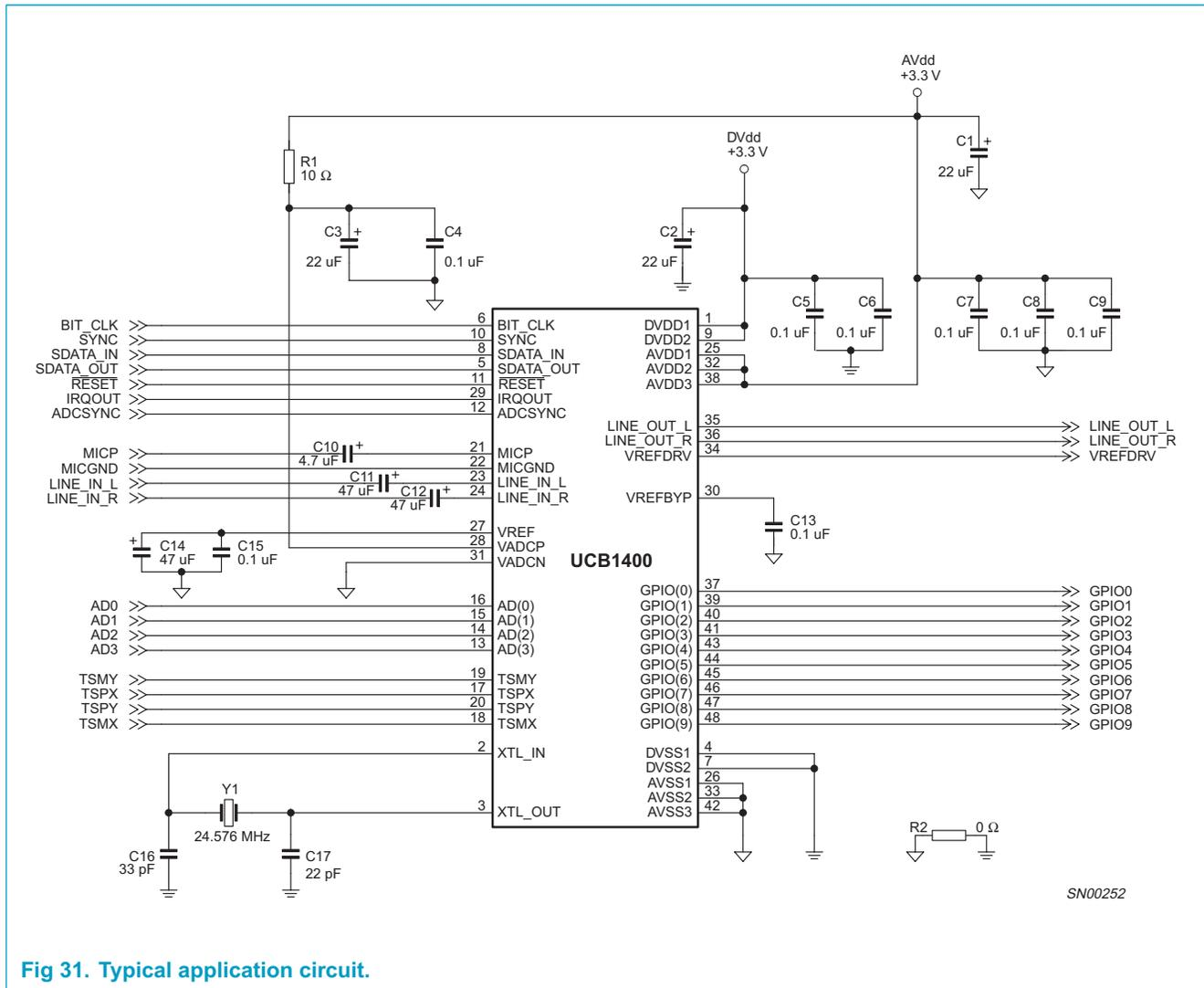
Fig 31. Typical application circuit.
