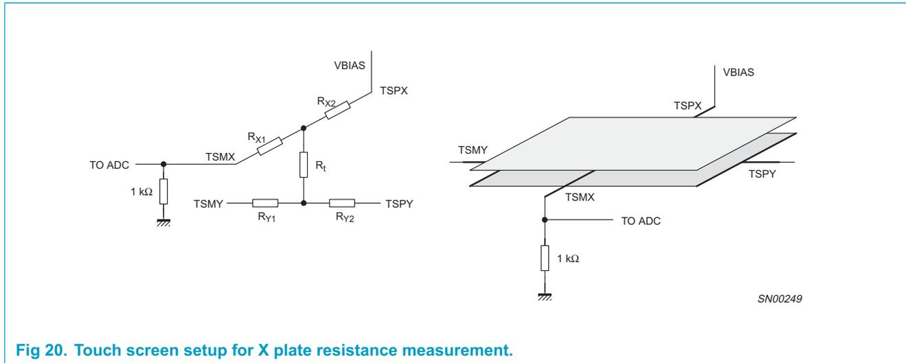
Fig 20. Touch screen setup for X plate resistance measurement.
