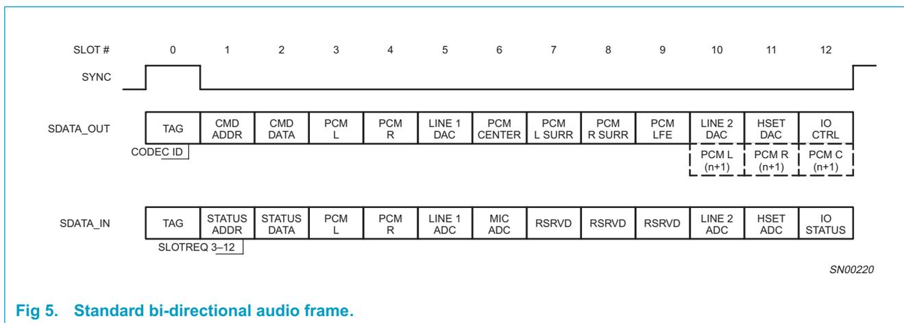
Fig 5. Standard bi-directional audio frame.
