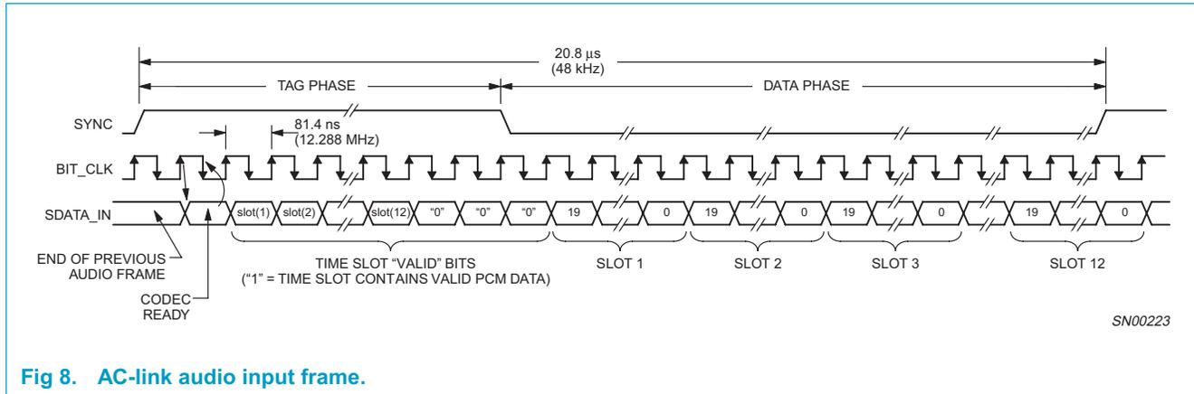
Fig 8. AC-link audio input frame.
