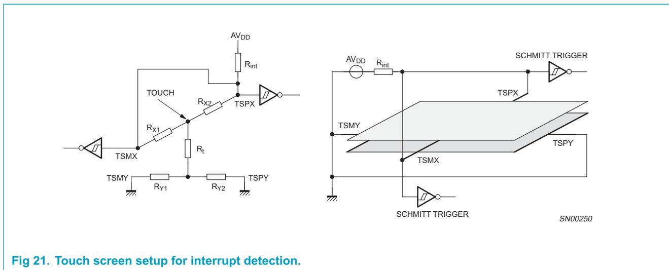
Fig 21. Touch screen setup for interrupt detection.
