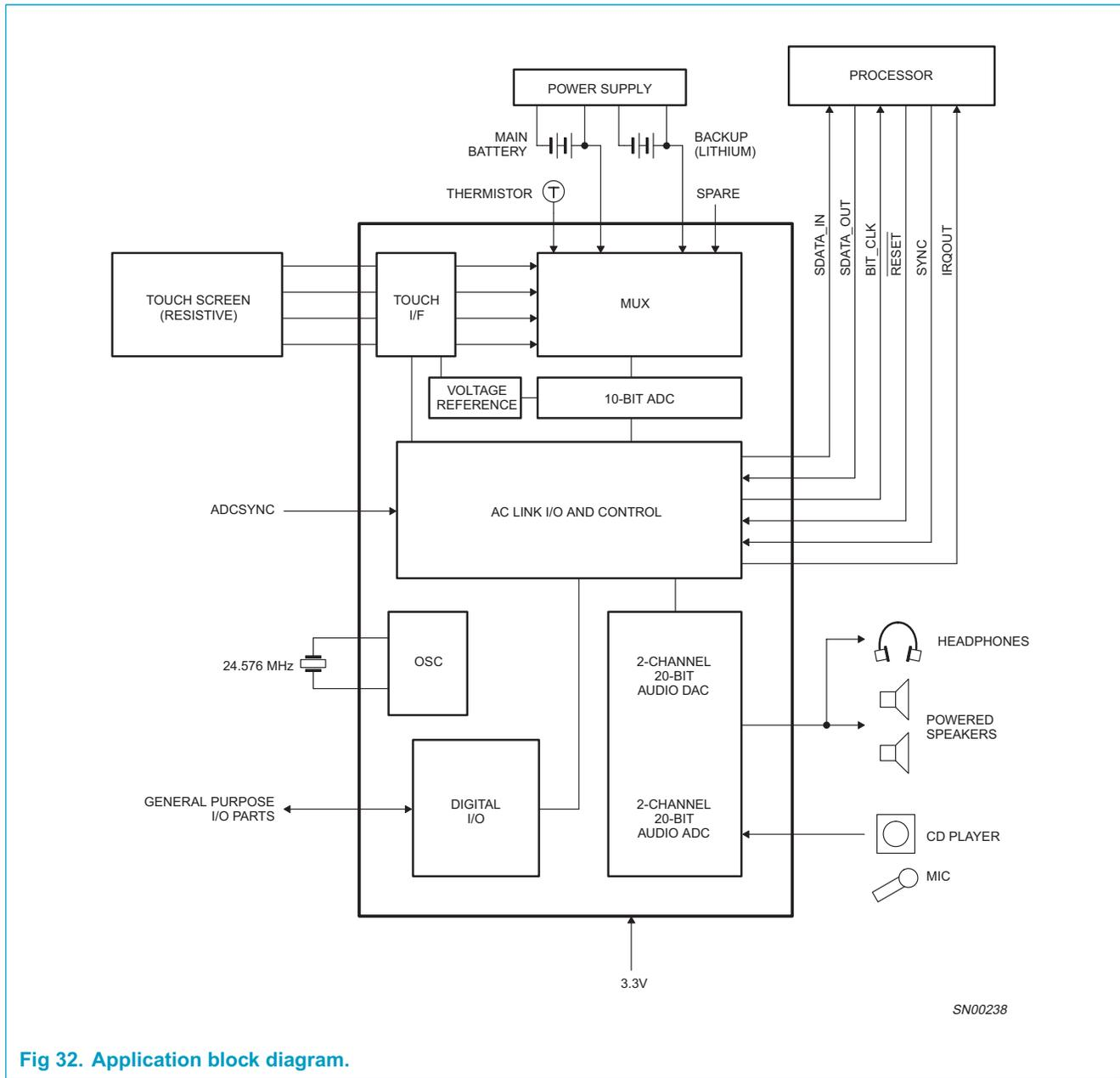
Fig 32. Application block diagram.
