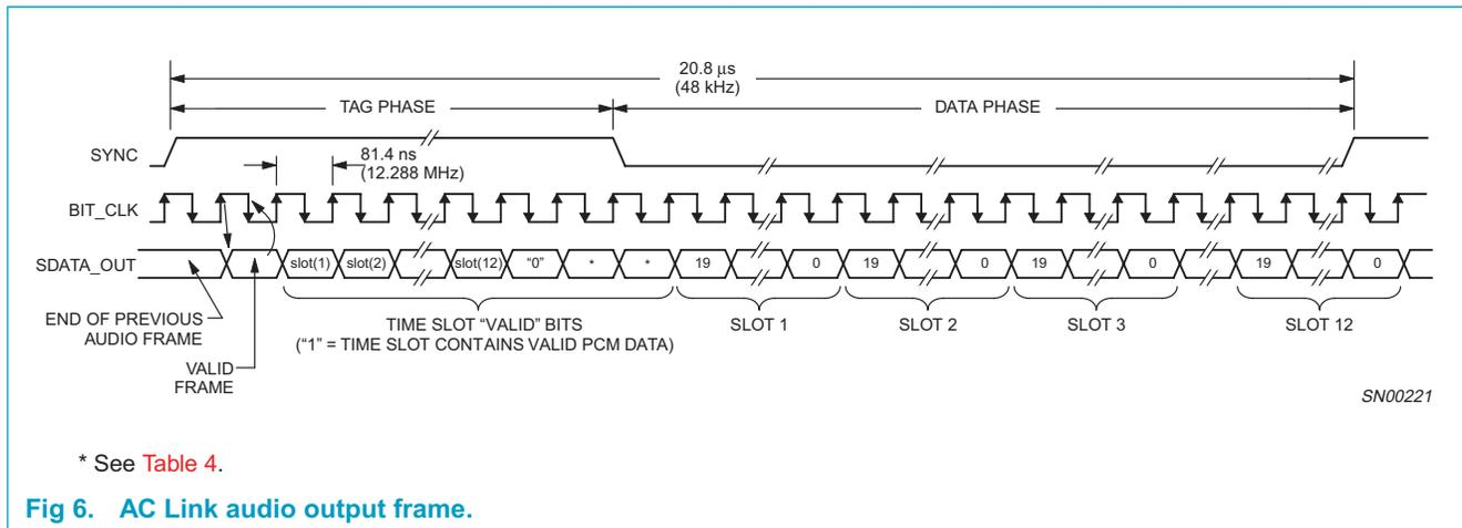
Fig 6. AC Link audio output frame.
