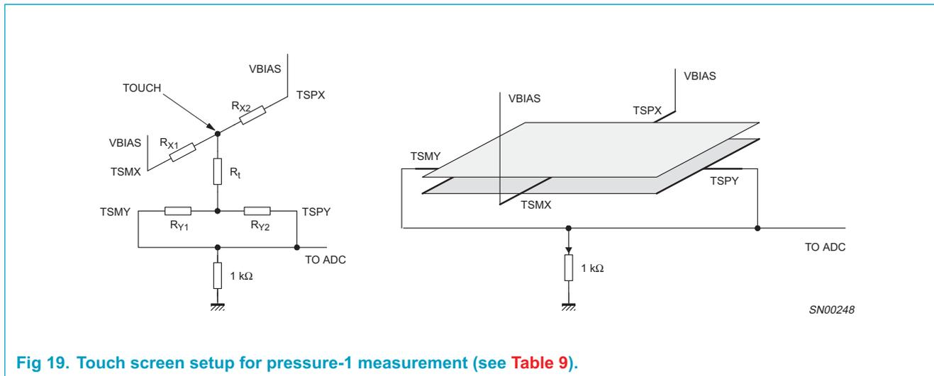
Fig 19. Touch screen setup for pressure-1 measurement (see Table 9).
