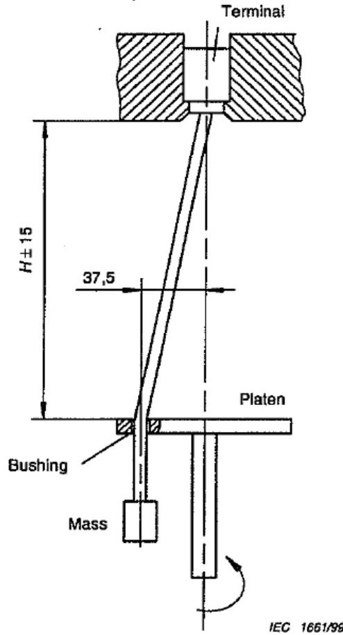
Figure 1 – Test apparatus according to 9.4
