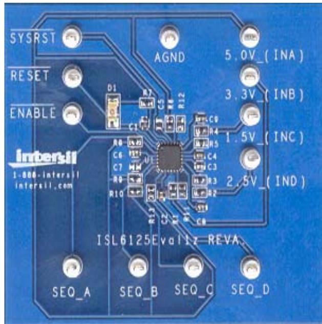
FIGURE 18. ISL6125EVAL1Z SCHEMATIC AND PHOTOGRAPH
