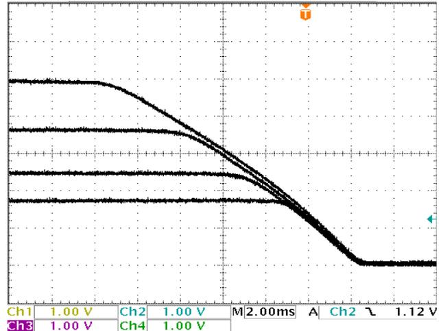
FIGURE 23. OUTPUT VOLTAGE ON HIGH TO LOW TRACKING
