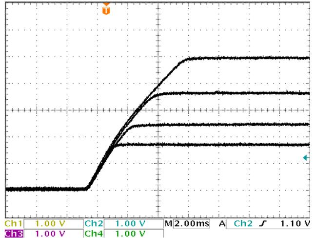
FIGURE 22. OUTPUT VOLTAGE ON LOW TO HIGH TRACKING
