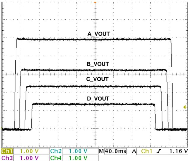
FIGURE 15. ISL6127 PRE-PROGRAMMED ABCD TURN-ON AND DCBA TURN-OFF
