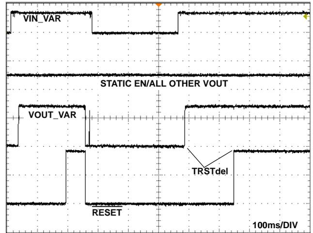
FIGURE 14. ISL6126 UVLO INPUT/OUTPUT INDEPENDENCE AND RESET RELATIONSHIP
