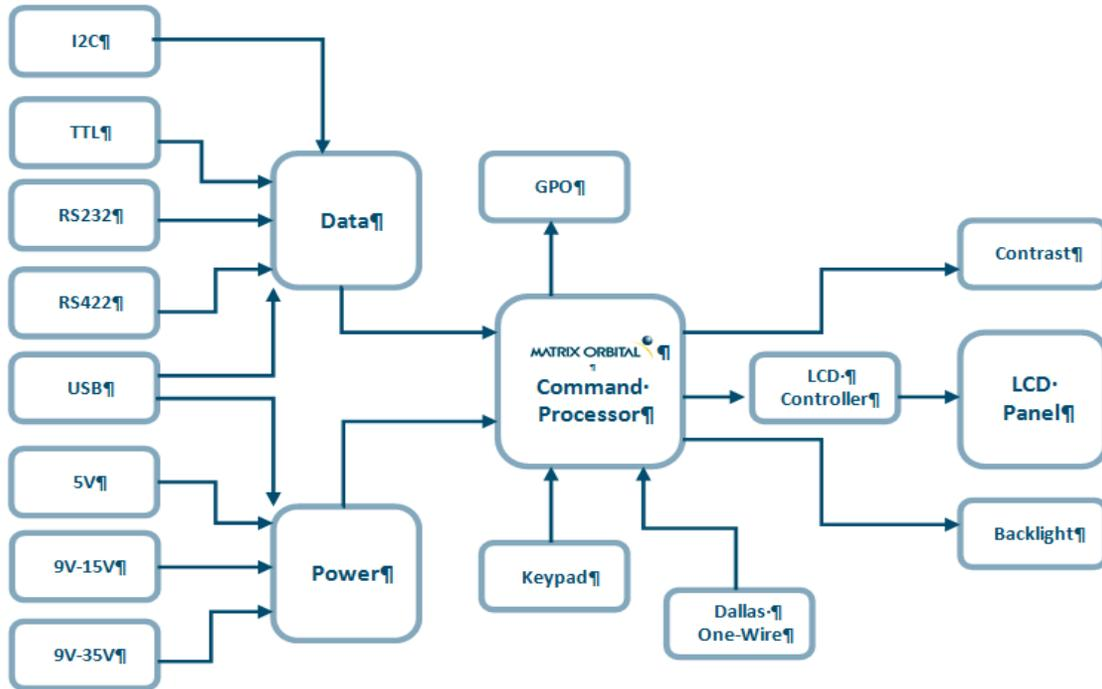
Figure 21: Functional Diagram
