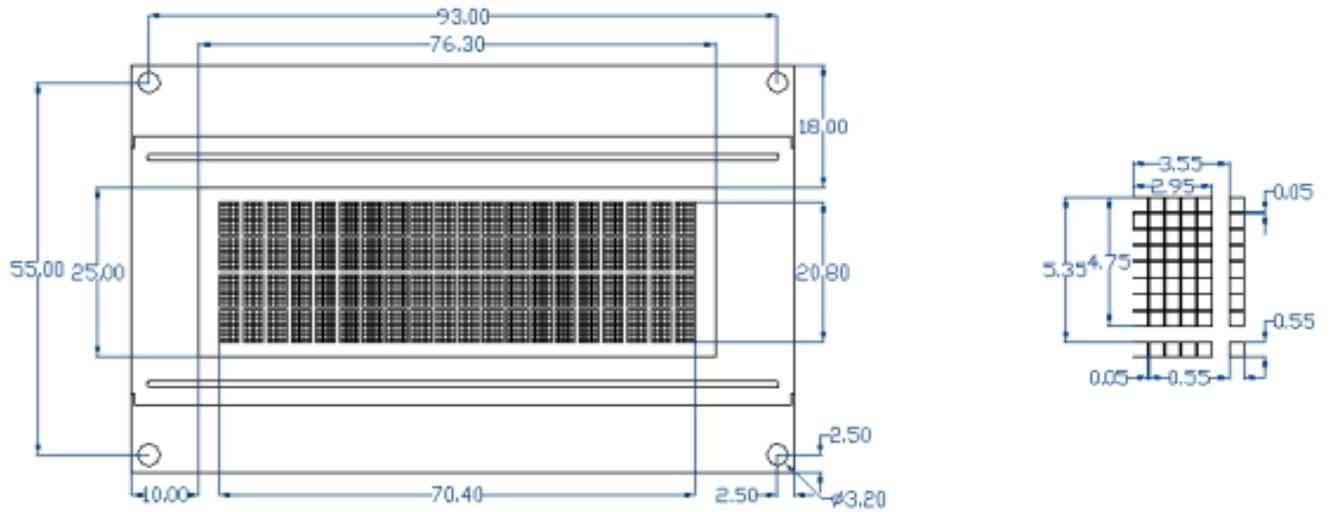
Figure 22: LCD Dimensional Drawing
