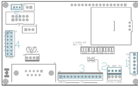
Figure 7: RS422 Connections
