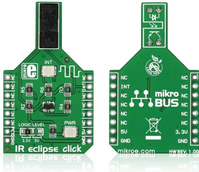
IR eclipse click™ carries an **EE-SX198** photo interrupter sensor. This sensor consists of an infrared transmitter and receiver facing each other and spaced apart by a 3mm slit. When the beam from the transmitter is eclipsed with by placing an object in the gap (like a piece of paper), the sensor is activated (indicated by the onboard INT LED). IR eclipse click™ communicates with the target board through the **mikroBUS™** INT line. It's designed to work with either a 3.3V or 5V power supply.
