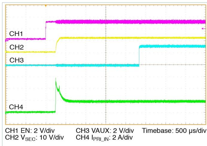
Figure 15 — Start up from application of EN with pre-applied  $V_{PRI\_DC} = 384 V$ , 50%  $I_{SEC\_DG}$ , 100%  $C_{SEC\_OUT\_EXT}$
