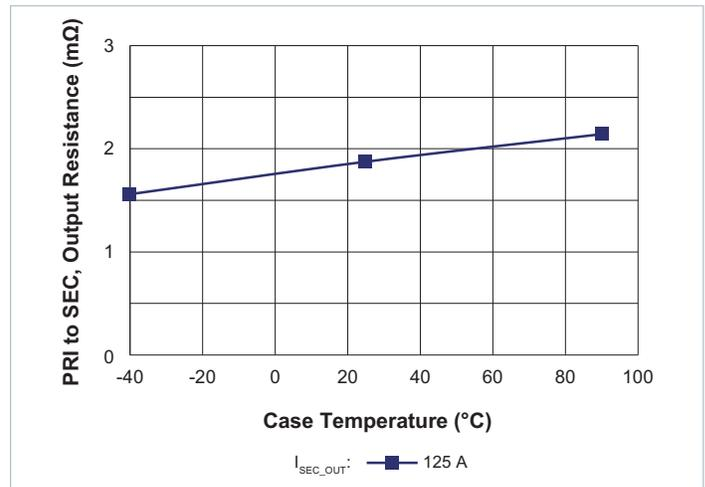
Figure 9 —  $R_{SEC}$  vs. temperature; Nominal  $V_{PRI\_DC}$
