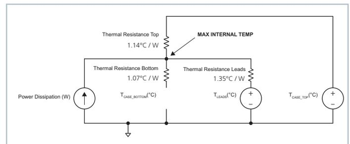
Figure 20 — Top case and leads thermal model
