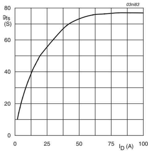
$T_j = 25^\circ\text{C}; V_{DS} = 25\text{V}$
