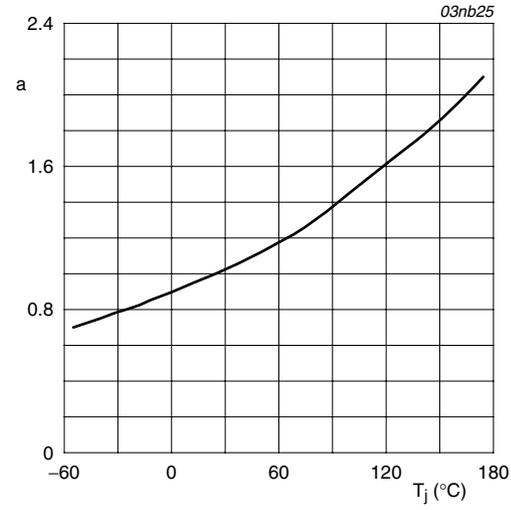
$$a = \frac{R_{DSon}}{R_{DSon(25^\circ\text{C})}}$$
