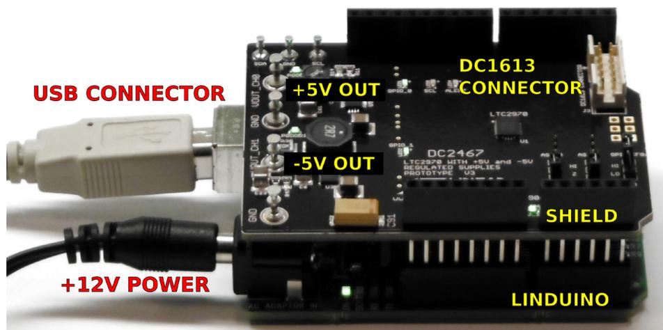
Figure 1. DC2467 Shield Mounted on the DC2026 Linduino
