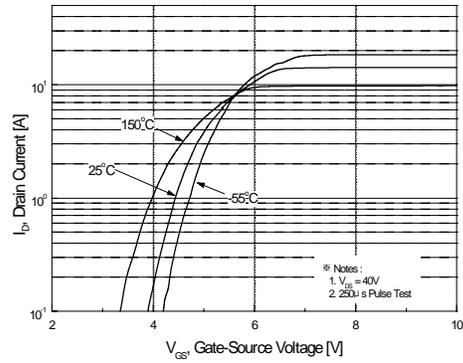
Figure 2. Transfer Characteristics
