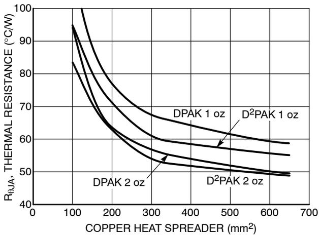
**Figure 22. Thermal Resistance vs. PCB Copper Area**
