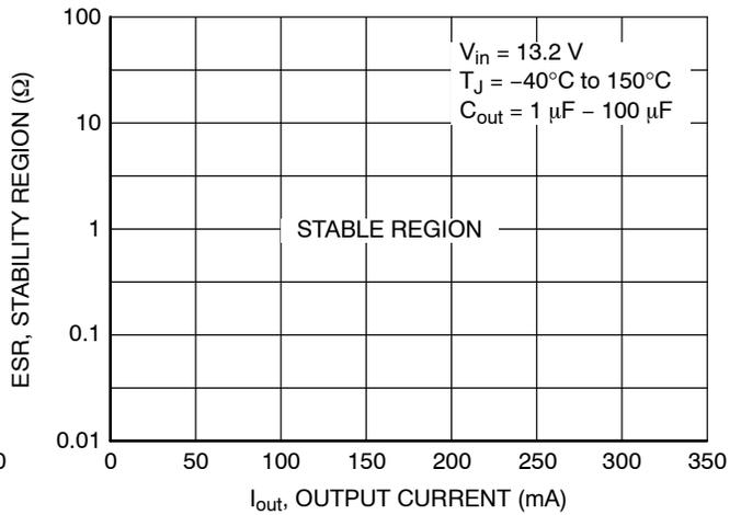
Figure 13. C<sub>out</sub> ESR Stability Region vs. Output Current
