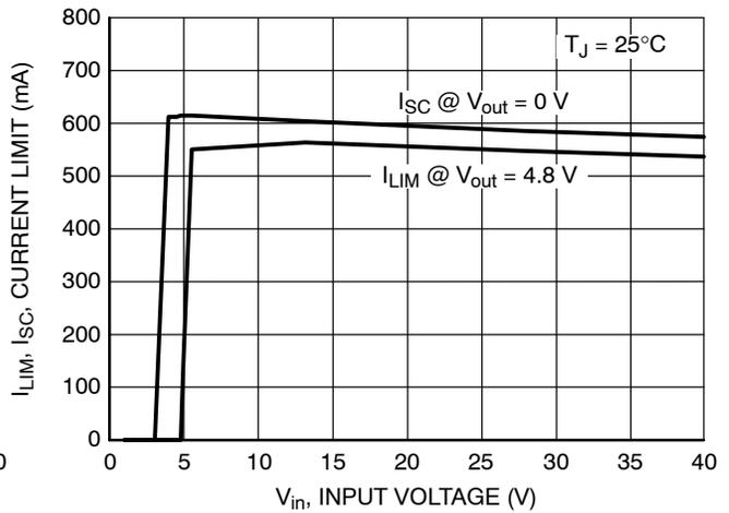
Figure 11. Output Current Limit vs. Input Voltage
