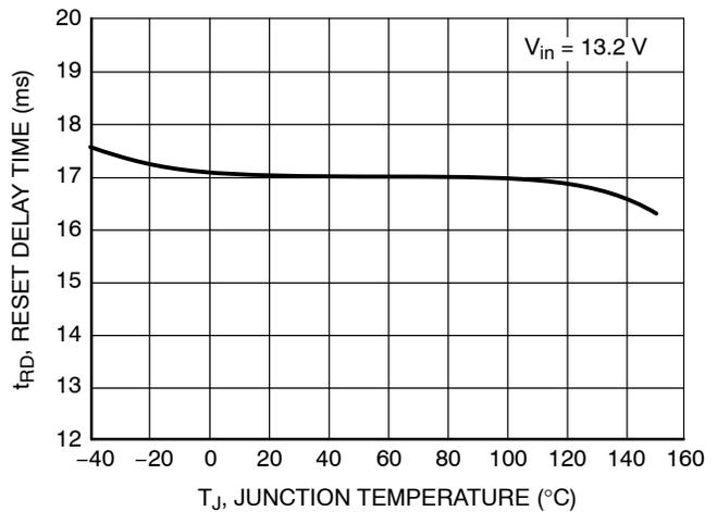
Figure 20. Reset Delay Time vs. Temperature
