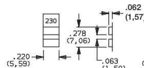
**13** SCREWDRIVER SLOT (WITHOUT MARKING)
