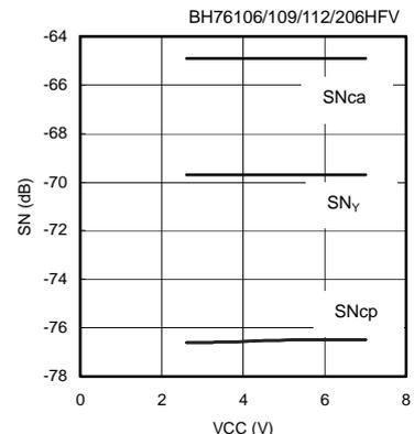
Fig.25 Supply Voltage-S/N
