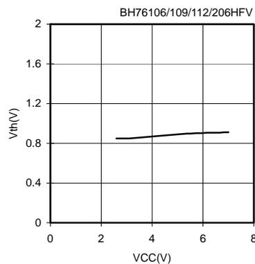
Fig.27 Supply Voltage-V<sub>th</sub>
