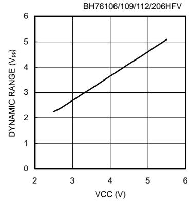
Fig.19 Dynamic Range Characteristic (VCC Characteristic)
