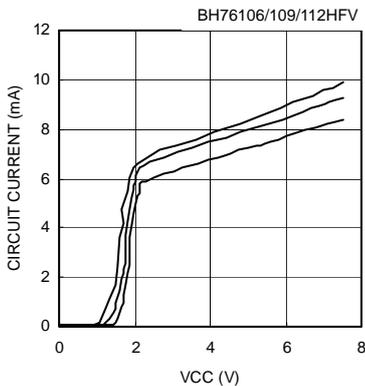
Fig.14 Supply Voltage-Circuit Current
