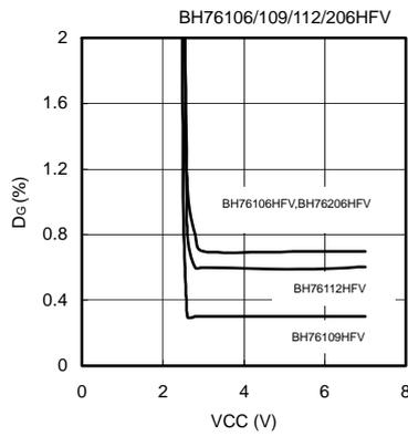
Fig.21 Supply Voltage-D<sub>G</sub>
