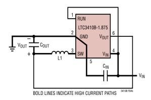
Figure 4b. LTC3410B-1.875 Layout Diagram
