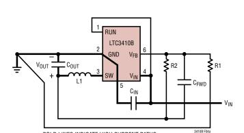
Figure 4a. LTC3410B Layout Diagram
