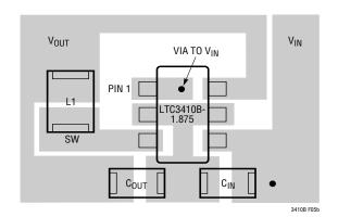
Figure 5b. LTC3410B Fixed Output Voltage Suggested Layout
