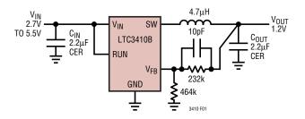
Figure 1. High Efficiency Step-Down Converter
