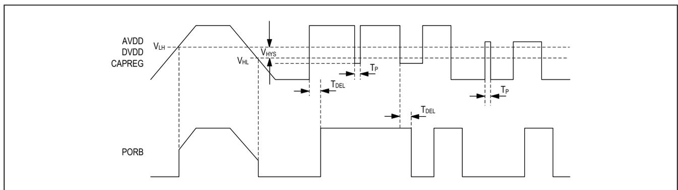
Figure 10. Undervoltage Lockout Characteristic Voltage Levels and Timing
