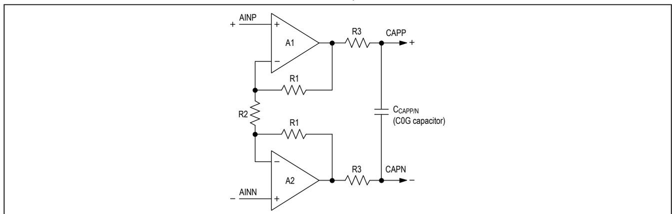
Figure 2. Simplified Equivalent Diagram of the PGA
