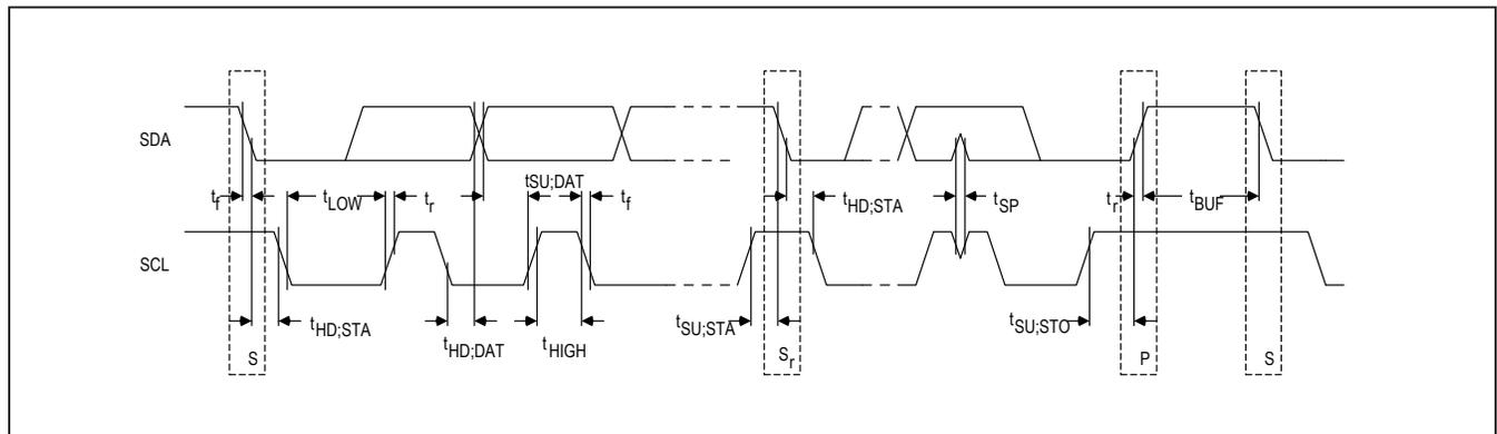
Figure 1. I<sup>2</sup>C Timing Diagram
