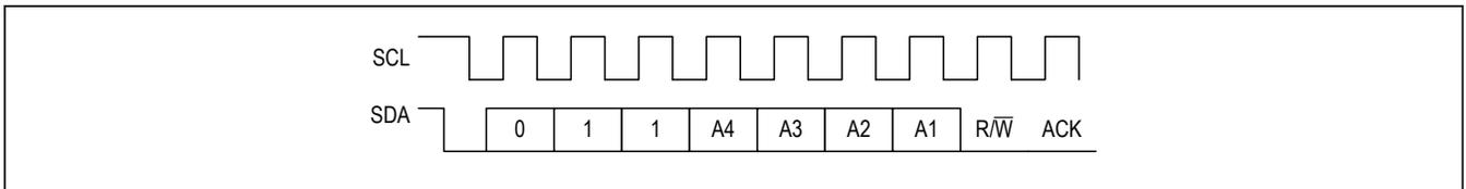
Figure 5. I<sup>2</sup>C Address Selection Byte Timing
