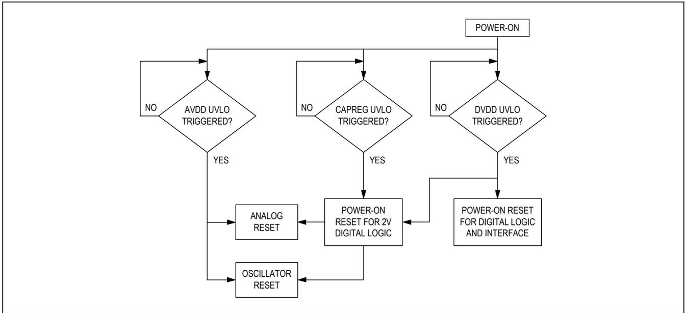
Figure 11. MAX11259 UVLO and POR Flow Diagram
