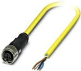
Sensor/Actuator cable, 4-position, TPE, yellow RAL 1021, free cable end, on Socket straight M12 SPEEDCON, A-coded, Cable length: 2 m
