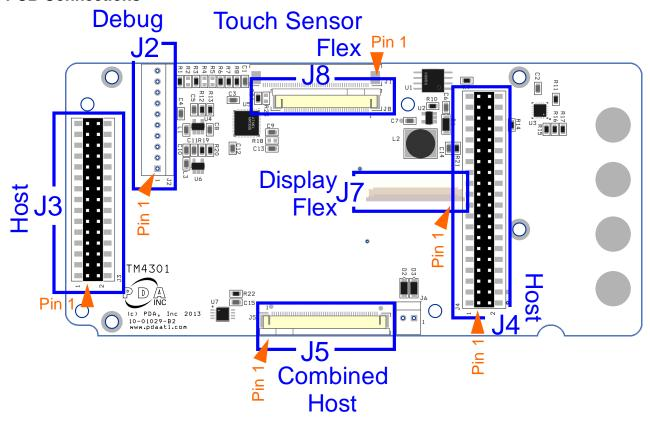
Figure 1 - PCB Connectors
