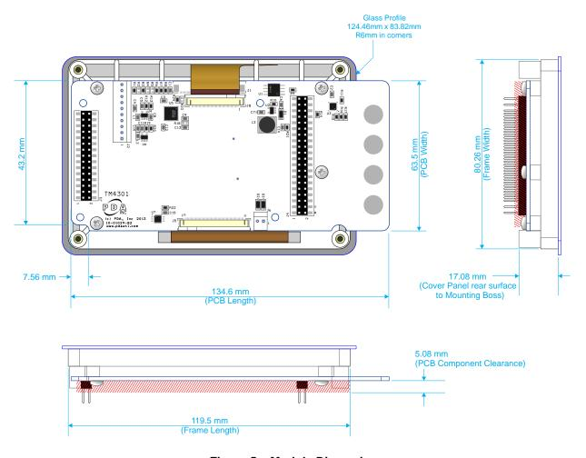
Figure 5 - Module Dimensions
