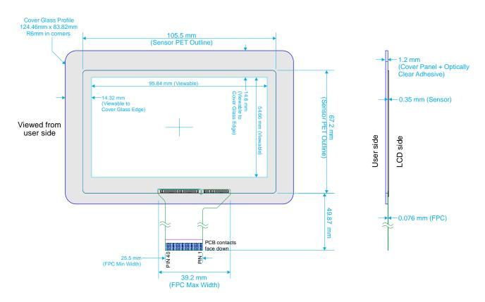
Figure 4 - Sensor Only Dimensions
