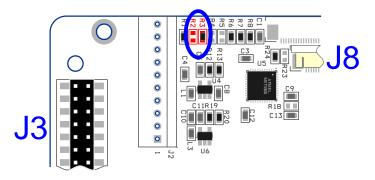
Figure 3 - Touch Controller I<sup>2</sup>C Address Selection
