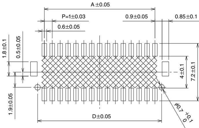
Note 1: Shaded area must be free of any electrically conductive traces to avoid contact with soldered pin header terminations.
