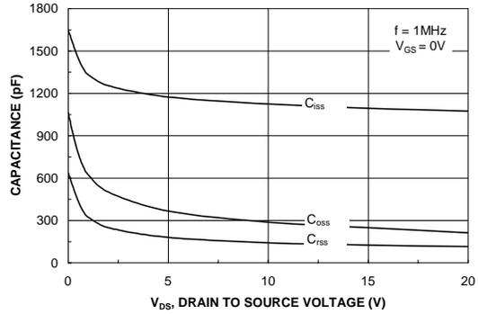
**Figure 8. Capacitance Characteristics**
