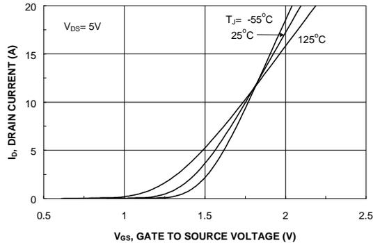
Figure 5. Transfer Characteristics.
