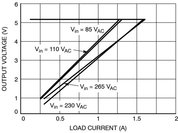
Figure 32. Converter Load Regulation
