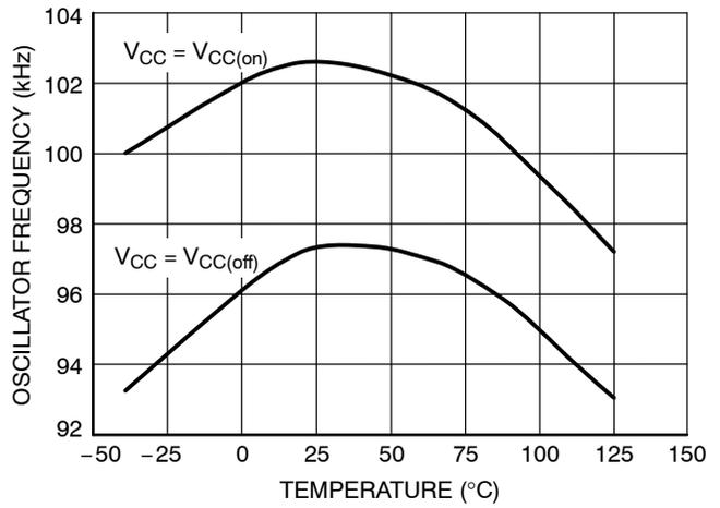
**Figure 6. Oscillator Frequency (100 kHz Version) versus Temperature**
