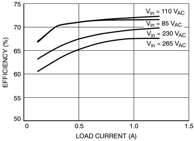
Figure 36. Converter Efficiency
