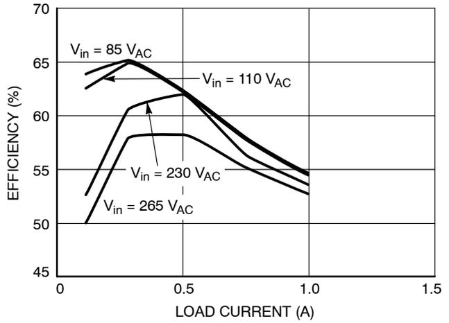
Figure 37. Charger Efficiency
