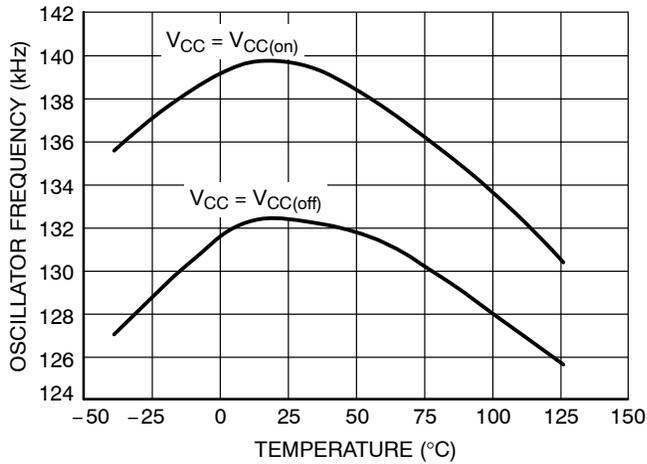
**Figure 7. Oscillator Frequency (136 kHz Version) versus Temperature**
