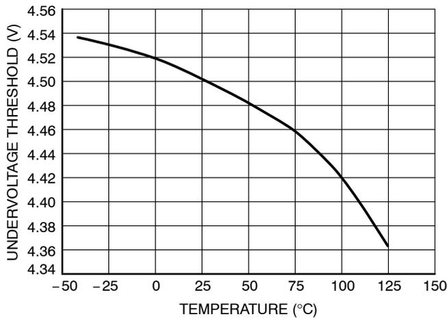
**Figure 19. Undervoltage Lockout Threshold versus Temperature**
