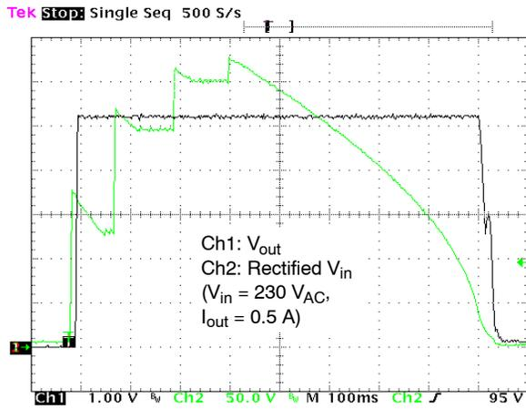
Figure 38. Converter On/Off Line Transient Response
