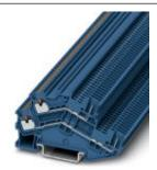
Multi-level terminal block, Cross section: 0.14 mm² - 1.5 mm², AWG: 26 - 14, Connection type: Push-in connection, Width: 3.5 mm, Color: blue, Mounting type: NS 35/7,5, NS 35/15
