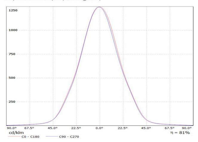
Luminaire: LEDiL Oy CN13114\_LENINA-M-DL\_(SoleriqE30) Lamps: 1 x Osram Soleriq E30 (1262.22lm@250mA)
