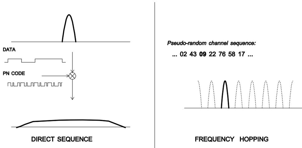
Forms of spread spectrum - direct sequence and frequency hopping
