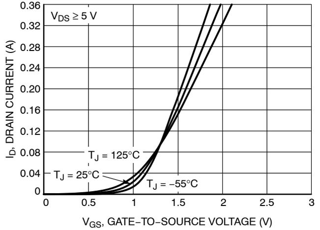
Figure 2. Transfer Characteristics
