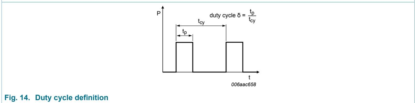
Fig. 14. Duty cycle definition
