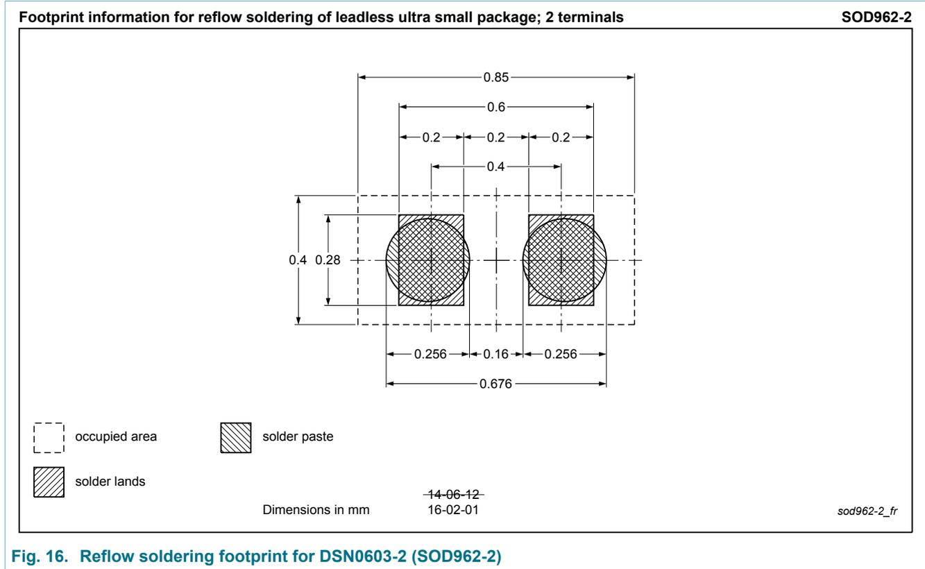
Fig. 16. Reflow soldering footprint for DSN0603-2 (SOD962-2)
