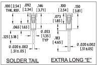
"A"= NO. OF PINS PER ROW x 0.100 [2.54] "B"= (NO. OF PINS PER ROW -1) x 0.100 [2.54]
