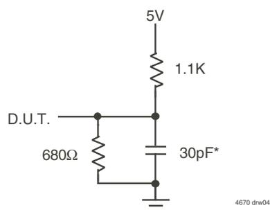
Figure 2. Output Load
