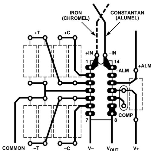
Figure 3. PCB Connections
