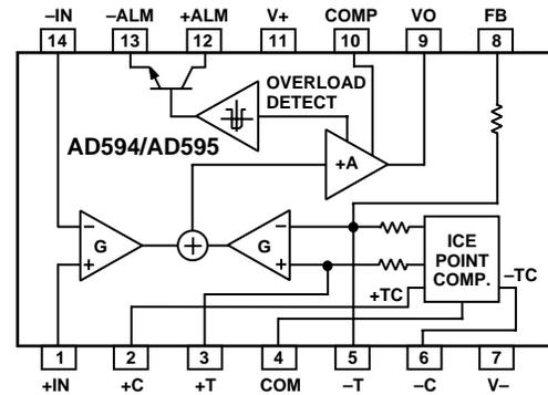
are available at the package pins so that the circuit can be recalibrated for the thermocouple types by the addition of two or three resistors. These terminals also allow more precise calibration for both thermocouple and thermometer applications.
