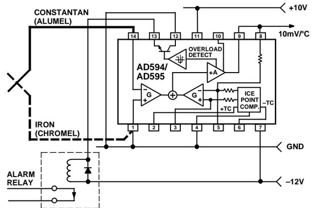
Figure 12.  $-ALM$  Driving A Negative Referenced Load
