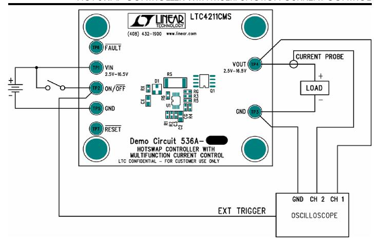
Figure 1. Test Setup of the DC536.
