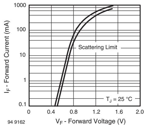
Fig. 2 - Forward Current vs. Forward Voltage
