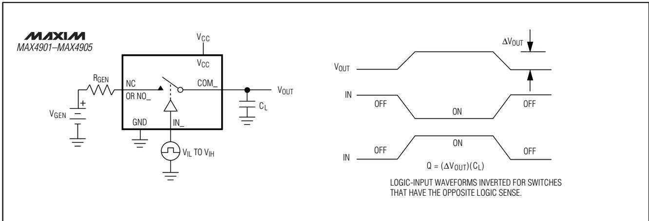
Figure 3. Charge Injection
