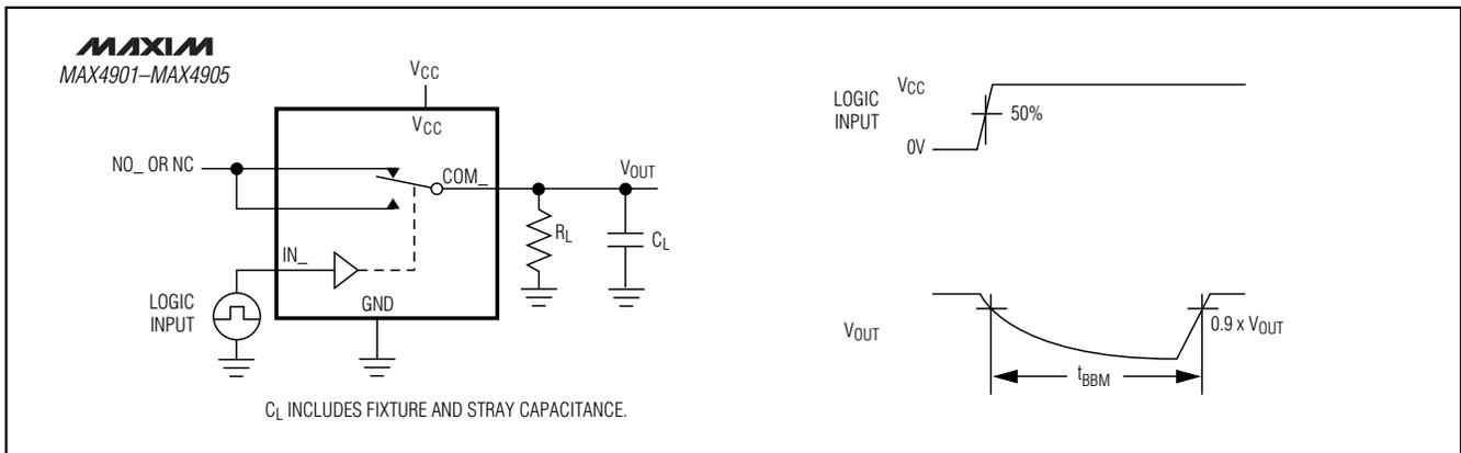
Figure 2. Break-Before-Make Interval
