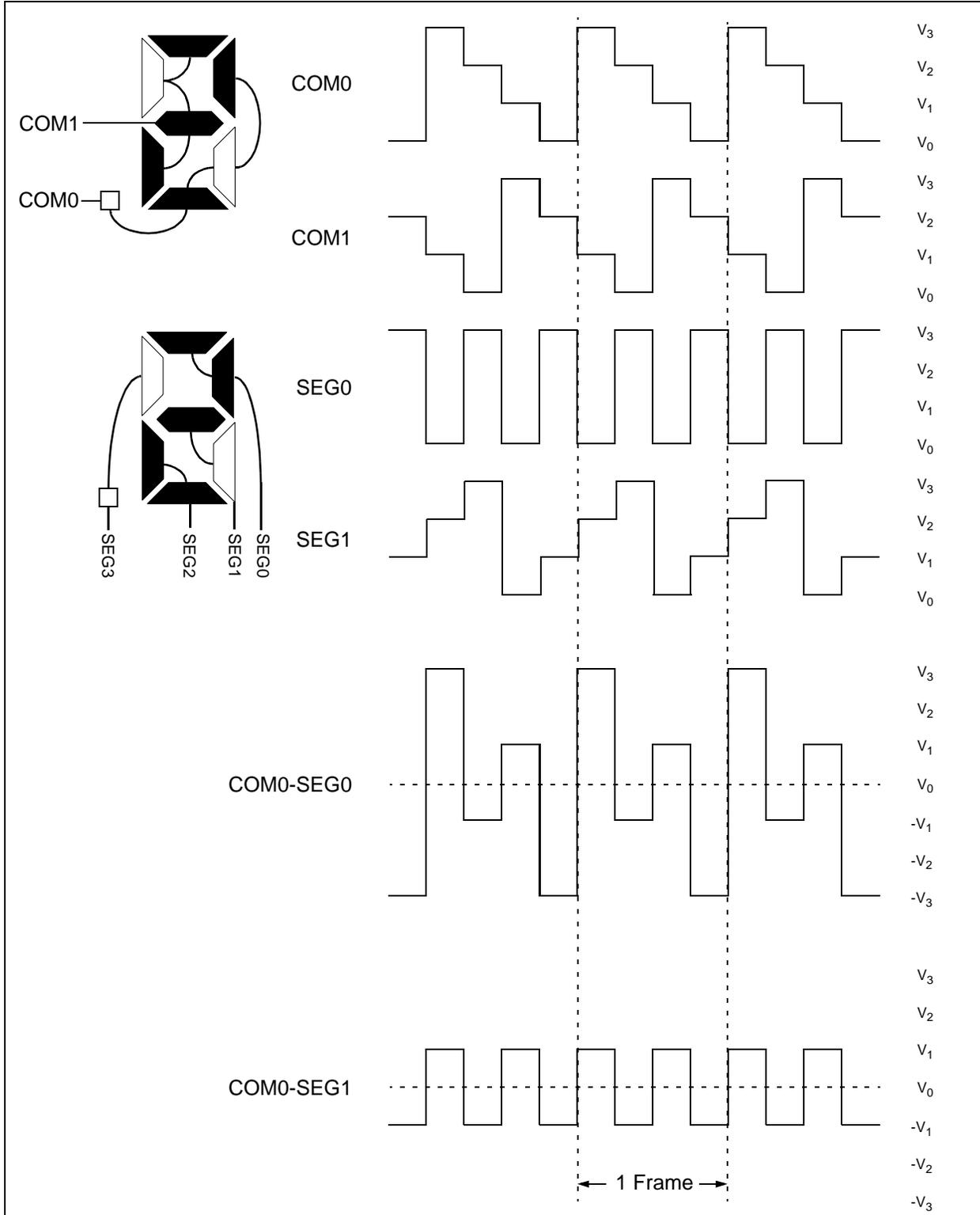
**FIGURE 11-4: WAVEFORMS IN 1/3 MUX, 1/3 BIAS**
