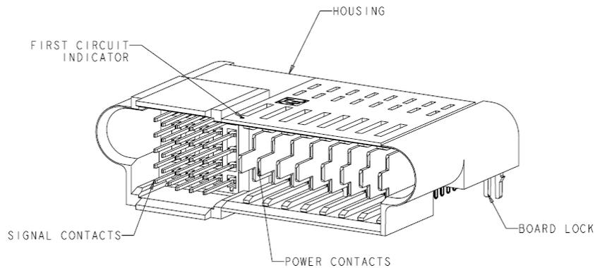
Front Connector View Looking at Blades and Pins (view looking in at rear of power supply)
