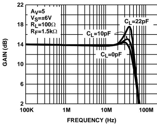
FIGURE 5. DIFFERENTIAL FREQUENCY RESPONSE vs  $C_L$  (EL1509CS)
