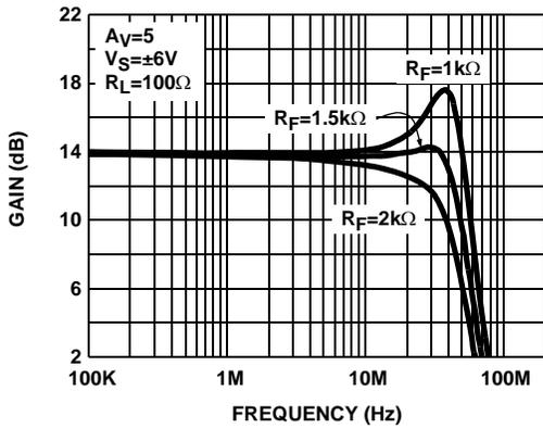
FIGURE 3. DIFFERENTIAL FREQUENCY RESPONSE vs  $R_F$  (EL1509CS)
