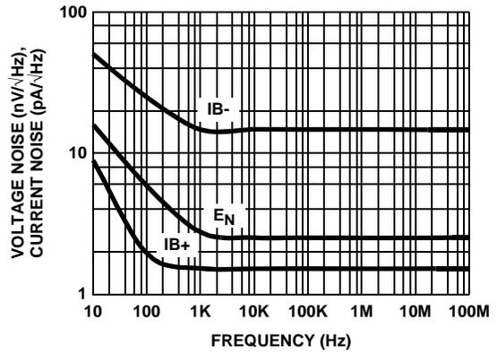
FIGURE 14. VOLTAGE AND CURRENT NOISE vs FREQUENCY
