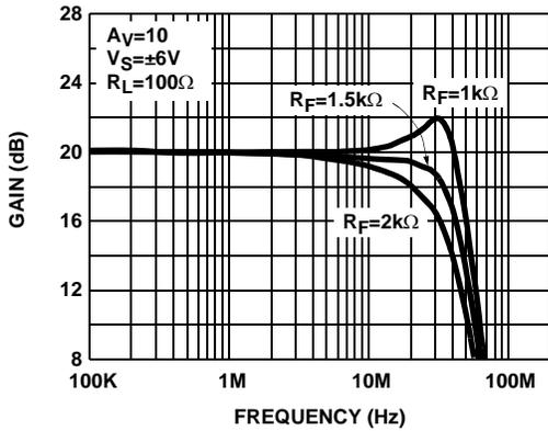
FIGURE 1. DIFFERENTIAL FREQUENCY RESPONSE vs  $R_F$  (EL1509CS)
