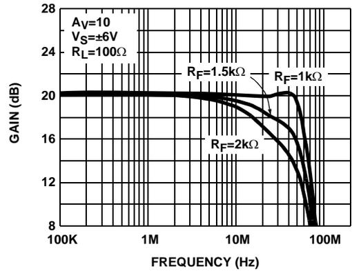
FIGURE 2. DIFFERENTIAL FREQUENCY RESPONSE vs  $R_F$  (EL1509CL)
