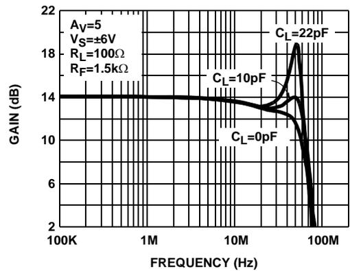
FIGURE 6. DIFFERENTIAL FREQUENCY RESPONSE vs  $C_L$  (EL1509CL)
