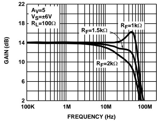
FIGURE 4. DIFFERENTIAL FREQUENCY RESPONSE vs  $R_F$  (EL1509CL)
