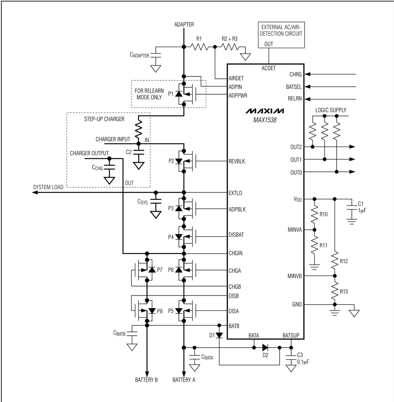
Figure 2. Typical Application Circuit for Step-Up/Step-Down Charger
