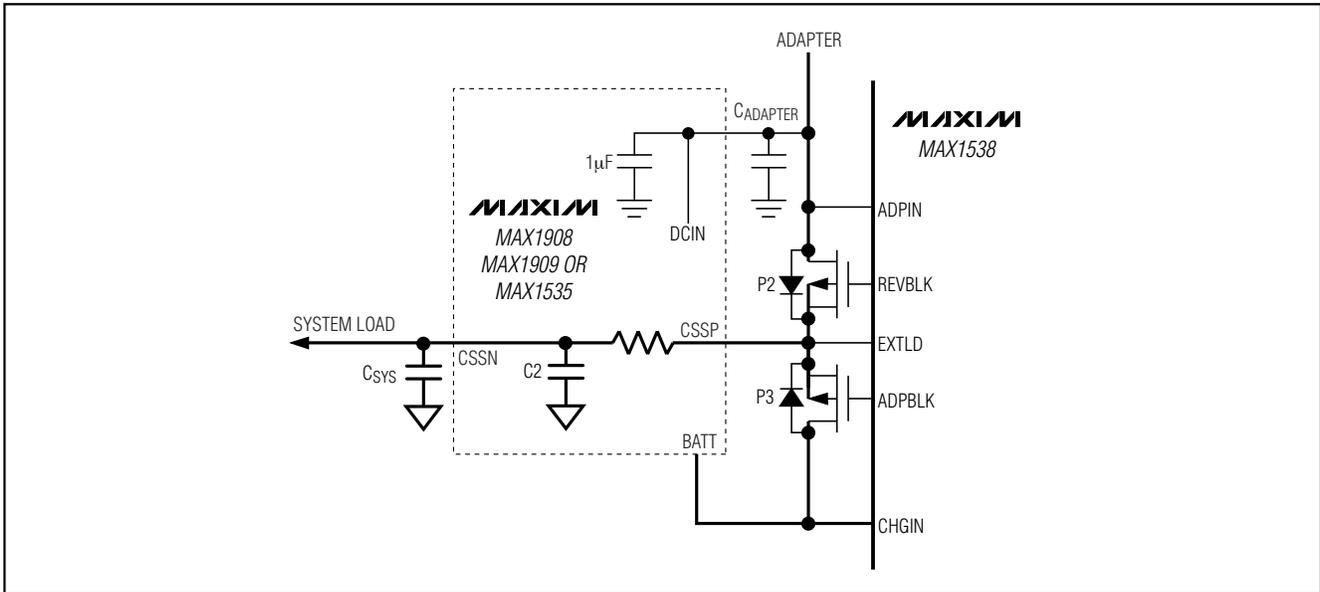
Figure 7. Combining the MAX1538 with a Charger
