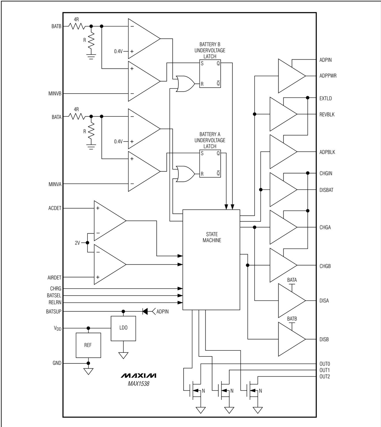
Figure 3. Functional Diagram
