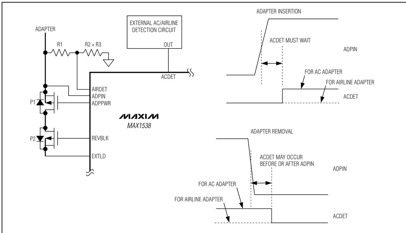
Figure 5. Using an External Adapter Detection Circuit
