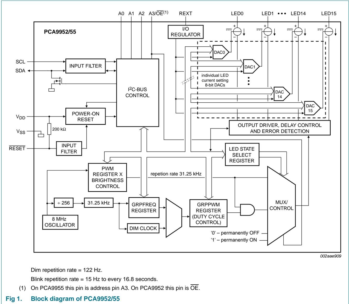
Fig 1. Block diagram of PCA9952/55
