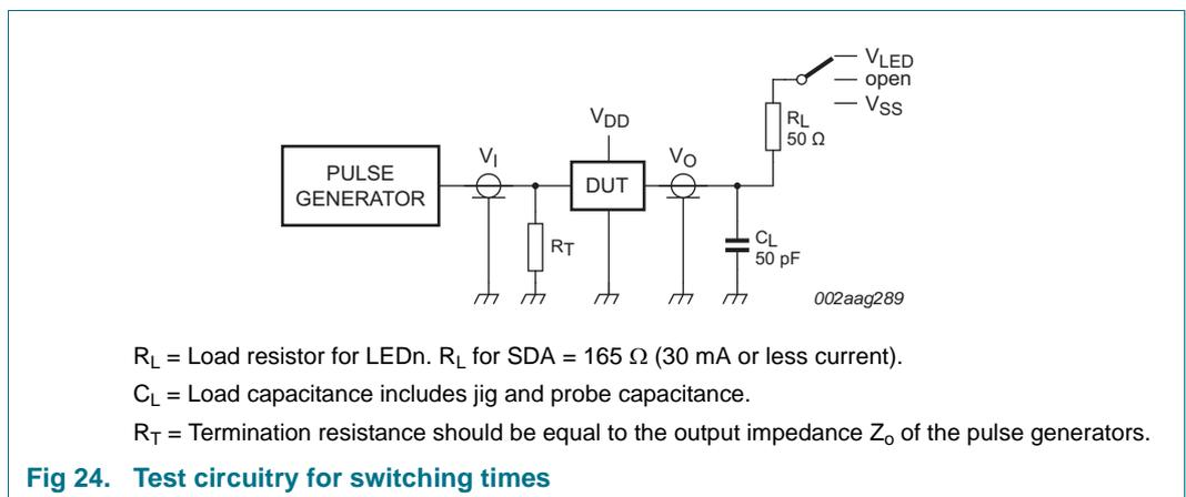
Fig 24. Test circuitry for switching times
