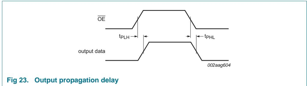
Fig 23. Output propagation delay
