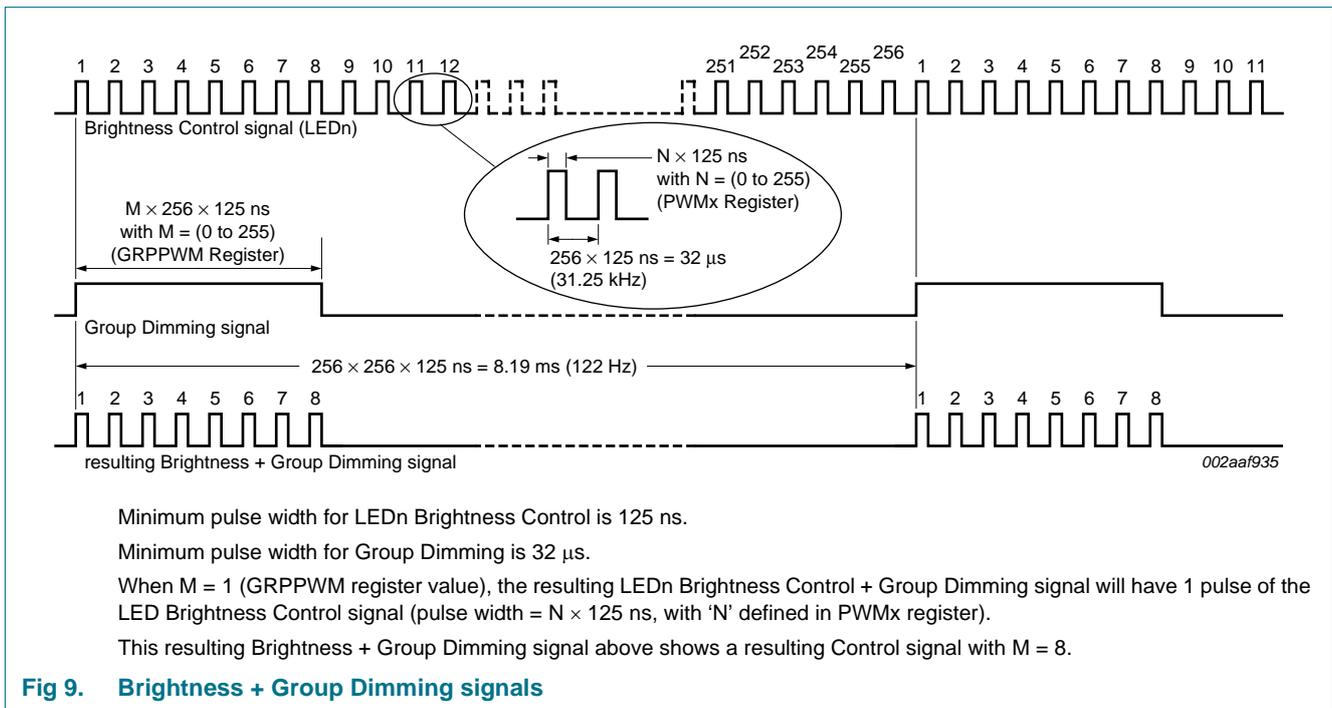
Fig 9. Brightness + Group Dimming signals
