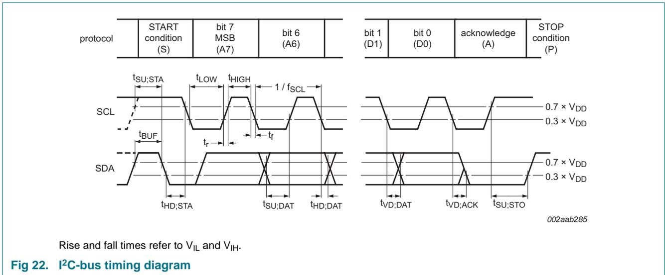
Fig 22. I<sup>2</sup>C-bus timing diagram
