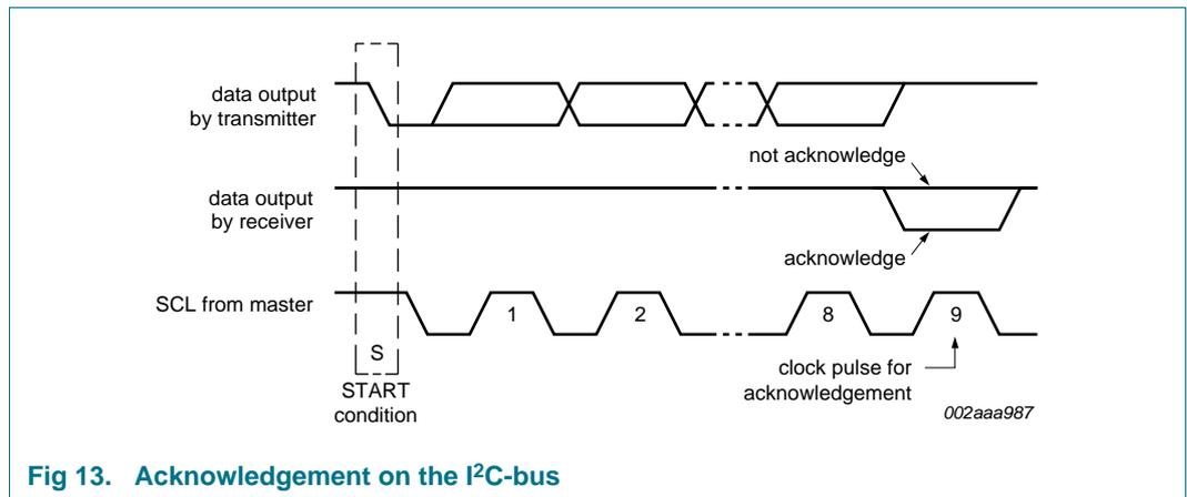
Fig 13. Acknowledgement on the I<sup>2</sup>C-bus
