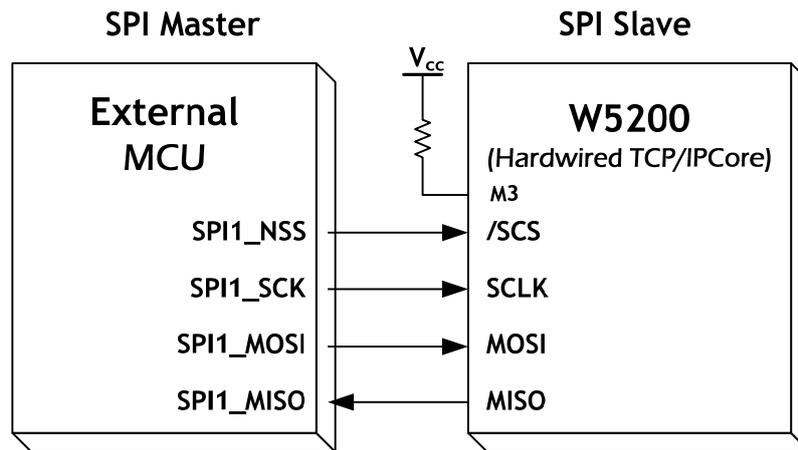
Figure 18 SPI Interface
