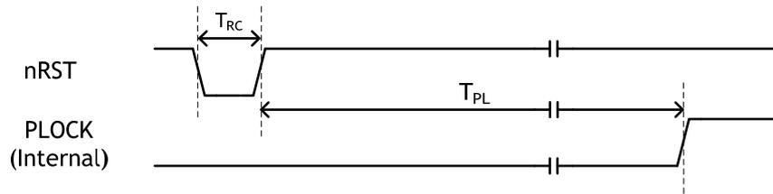
Figure 23 Reset Timing
