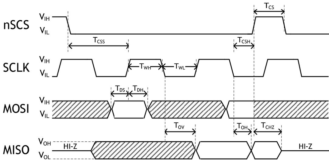
Figure 24 SPI Timing
