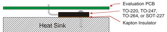
**Figure 2 - EVDD404 Side View Showing Power Device Installed In A High-Power Configuration**
