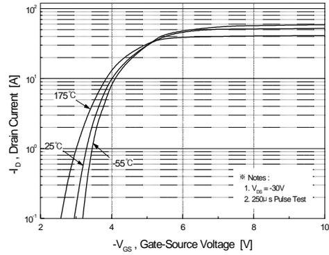
Figure 2. Transfer Characteristics
