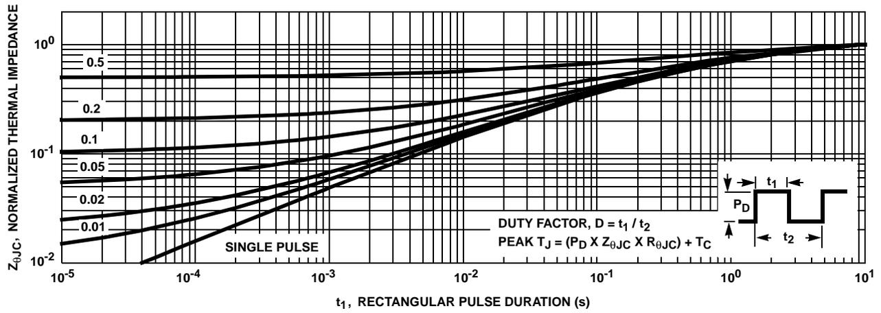
FIGURE 16. NORMALIZED TRANSIENT THERMAL RESPONSE, JUNCTION TO CASE
