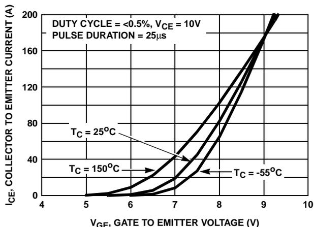
FIGURE 13. TRANSFER CHARACTERISTIC
