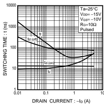
Fig.8 Switching Characteristics
