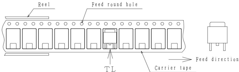
Those with one electrode terminal on the feed hole side.....TL
