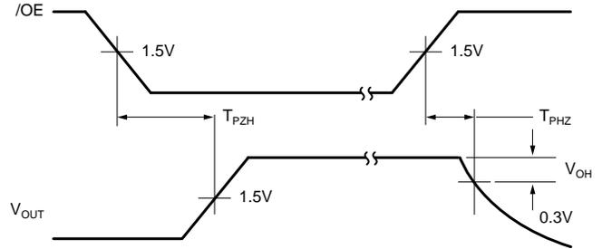
Figure 2. 3-State Output High Enable and Disable Times
