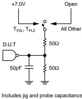
Figure 3. Test Load
