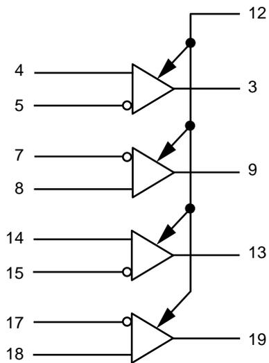
$V_{CC}$  (+5 VDC) = Pins 2 and 20; GND = Pin 10
