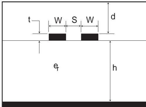
**Figure 11: Equations for the Differential Microstrip Construction:**
