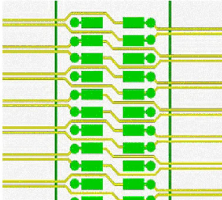
**Figure 38: Analyzer Probe Footprint**
