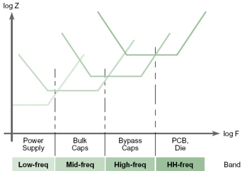
As the frequency changes, each part of the power distribution system responds proportionally; the low-impedance power supply responds to slow events, bulk capacitors to mid-frequency events, and so forth.
