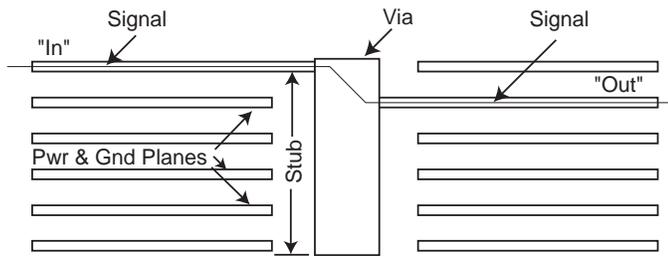
**Figure 18: Signal Through a Via**
