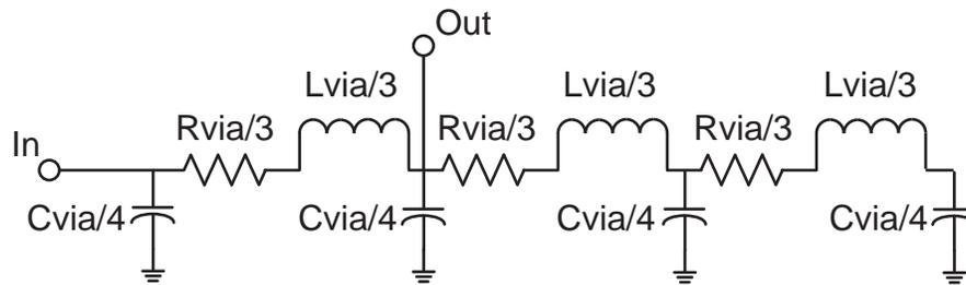
**Figure 20: Signal Transitioning Through a Via Simulation Model**
