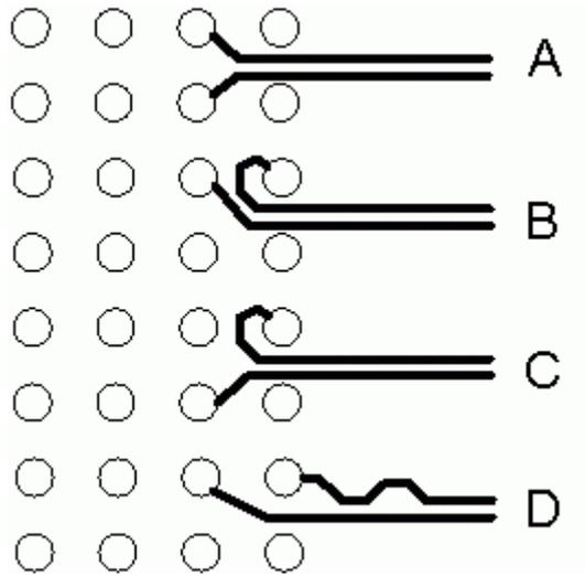
**Figure 26: Differential Skew Matching Serpentine**
