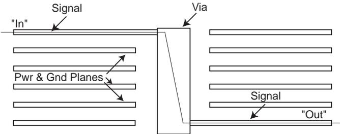
Because of the high frequencies present in the RapidIO signal, vias become a significant contributor to signal degradation. Most vias are formed by a cylinder going through the PCB board. Because the via has some length, there is an inductance associated with the via. Parasitic capacitance comes from the power and ground planes through which the via passes. From this structure, the model of the vias in RLC lumps as shown in [Figure 19](#) and [Figure 20](#).
