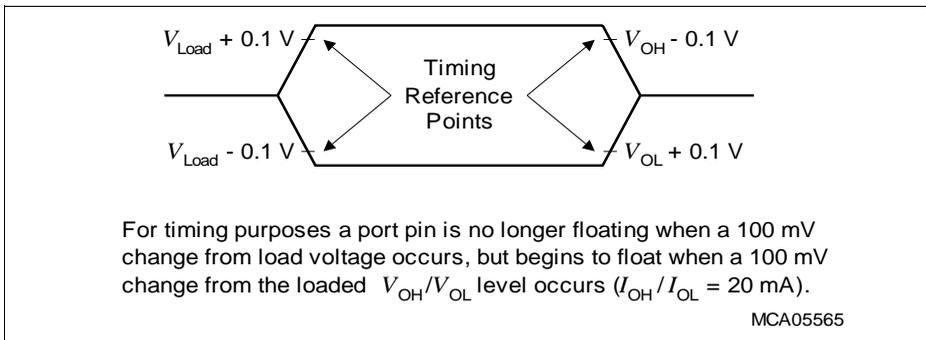
Figure 16 Floating Waveforms
