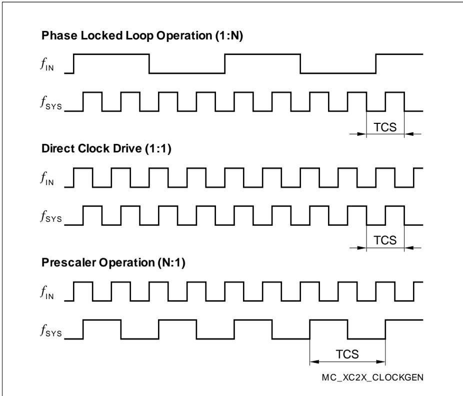
**Figure 17 Generation Mechanisms for the System Clock**
