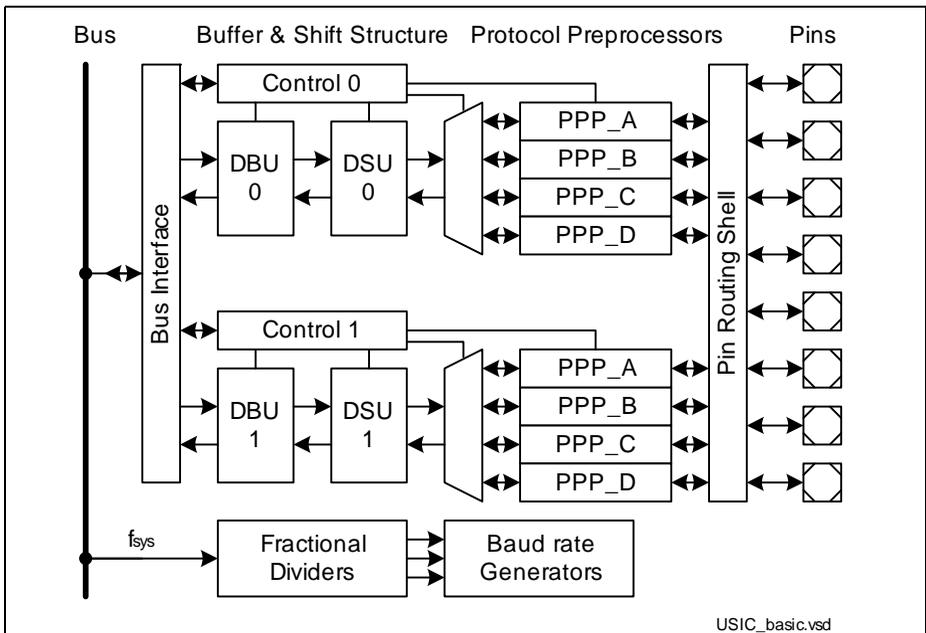
**Figure 10 General Structure of a USIC Module**
