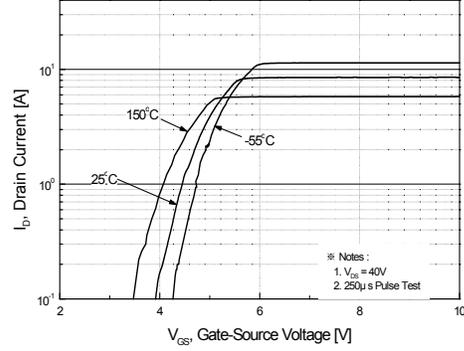
**Figure 2. Transfer Characteristics**
