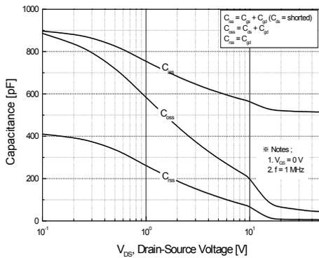
**Figure 5. Capacitance Characteristics**
