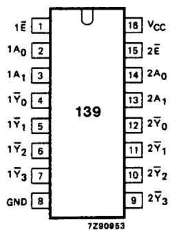
Fig.1 Pin configuration.
