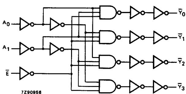
Fig.5 Logic diagram (one decoder/demultiplexer).
